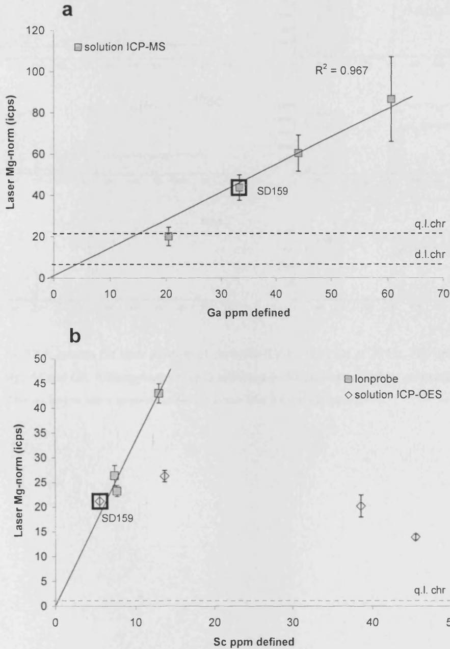
Figure 9: Signal intensity of the laser (intensity counts per second-icps) normalised to Mg against concentration of Ga (at 15Hz, 40  $\mu$ m), defined by solution ICP-MS, and Sc (at 20 Hz, 100  $\mu$ m) defined by ICP-OES and ionprobe. Solution prepared from bulk-rock powder (SD159) highlighted by open square whereas solutions prepared from microdrilled powder not highlighted. R2 - correlation coefficient, D.L- detection limit and Q.L.- quantification limit.
