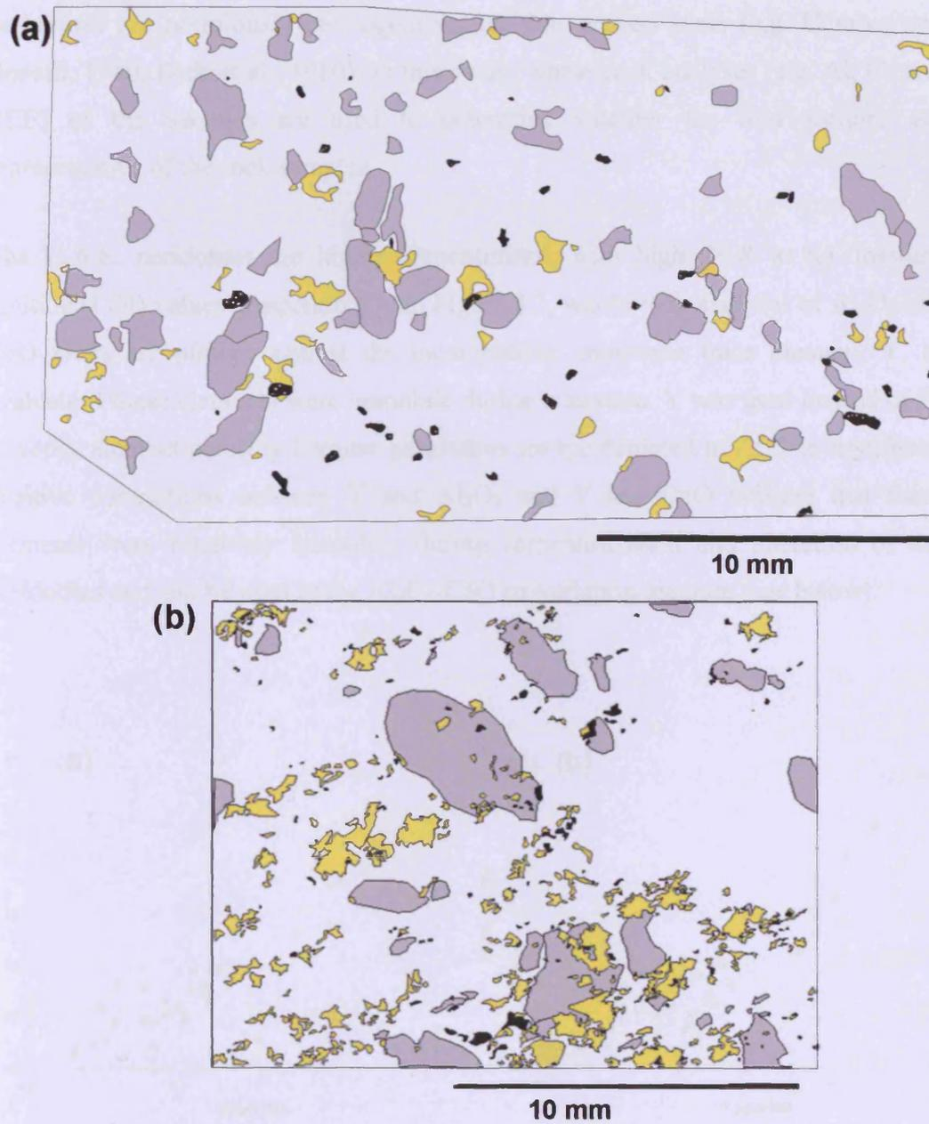
Figure 3.2: SEM image mapping of (a) **clinopyroxene-rich harzburgite** (U.A.E.327) and (b) **lherzolite** (U.A.E.2065). Orthopyroxene (grey), clinopyroxene (yellow), spinel (black) and olivine (white). The proportion of clinopyroxene is estimated as 4% in (a) and 13% in (b).
