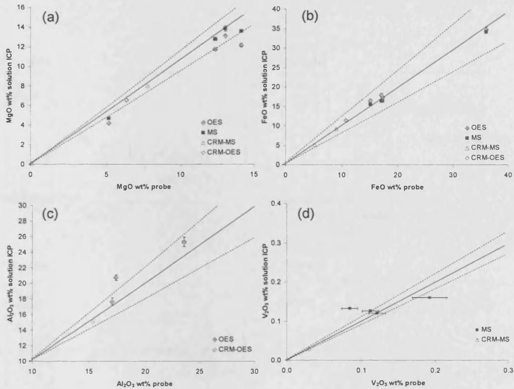
Figure 2: Comparison of element abundances determined by solution ICP-MS/OES and electron microprobe for (a) MgO, (b) FeO, (c) Al<sub>2</sub>O<sub>3</sub> and (d) V<sub>2</sub>O<sub>5</sub>. Solid line marks 1:1 correlation line and dashed lines mark ± 10% relative difference.
