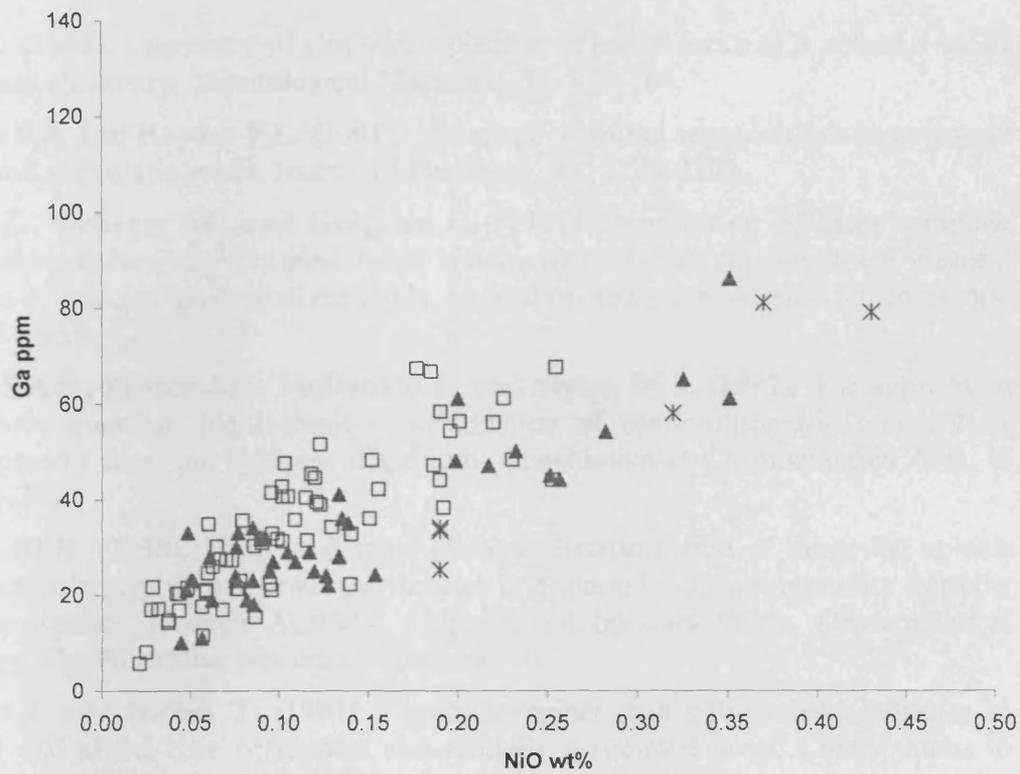
Figure 14: Comparison of Ga and Ni measured in chromites by proton microprobe (black triangles: O'Reilly et al. 1991, Ewart and Griffin 1994, Paktunc and Cabri 1995, Paktunc and Hulbert 1996), LA-ICP-MS using matrix-matched standards in chromites (open squares: Dare et al. 2007) and by LA-ICP-MS using NIST glass standards (crosses: Eggins et al., 1998, Norman 1998).
