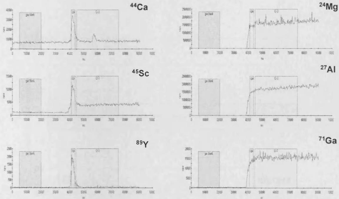
Figure 10: TRA spectra for laser ablation of chromite (Cr-3 = SD159) at 20 Hz, 100  $\mu\text{m}$  line width for Ca, Sc, Y, Mg, Al and Ga. Clinopyroxene (cpx) inclusion ( $\sim 10 \mu\text{m}$ ) identified by co-existing peaks in Ca, Sc and Y. The inclusion has a negligible deficit in the Mg, Al and Ga intensities.
