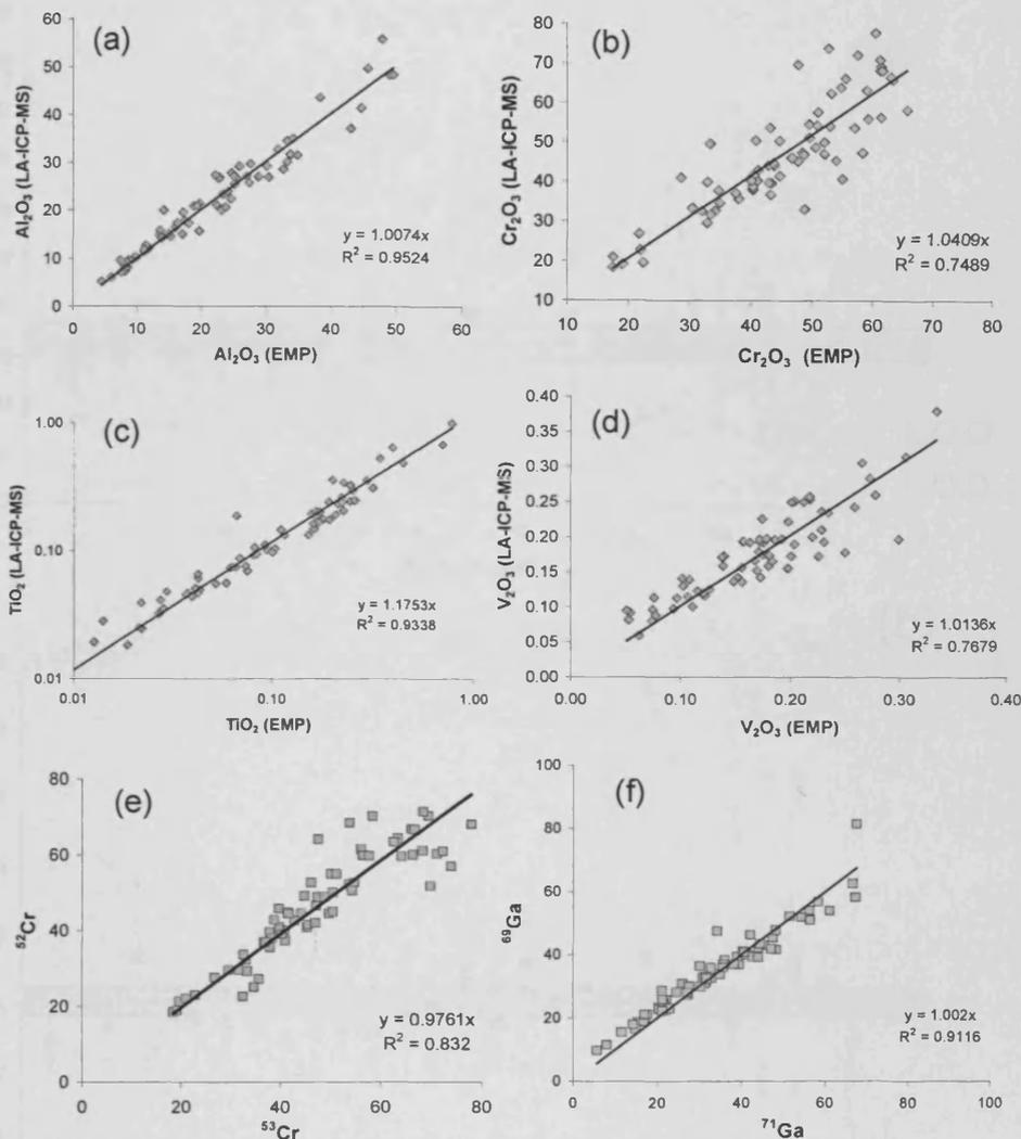
Figure 5.2: Comparison of laser-ablation ICP-MS and electron microprobe values for (a)  $\text{Al}_2\text{O}_3$ , (b)  $\text{Cr}_2\text{O}_3$ , (c)  $\text{TiO}_2$  and (d)  $\text{V}_2\text{O}_3$  show good agreement (1:1 relationship) between LA-ICP-MS and EMP data for chrome-spinels. Comparison between two isotopes measured simultaneously for Cr (e) and Ga (f) show good agreement (1:1) but low  $r^2$ , particularly for Cr partly because of erratic interference on  $^{52}\text{Cr}$ .
