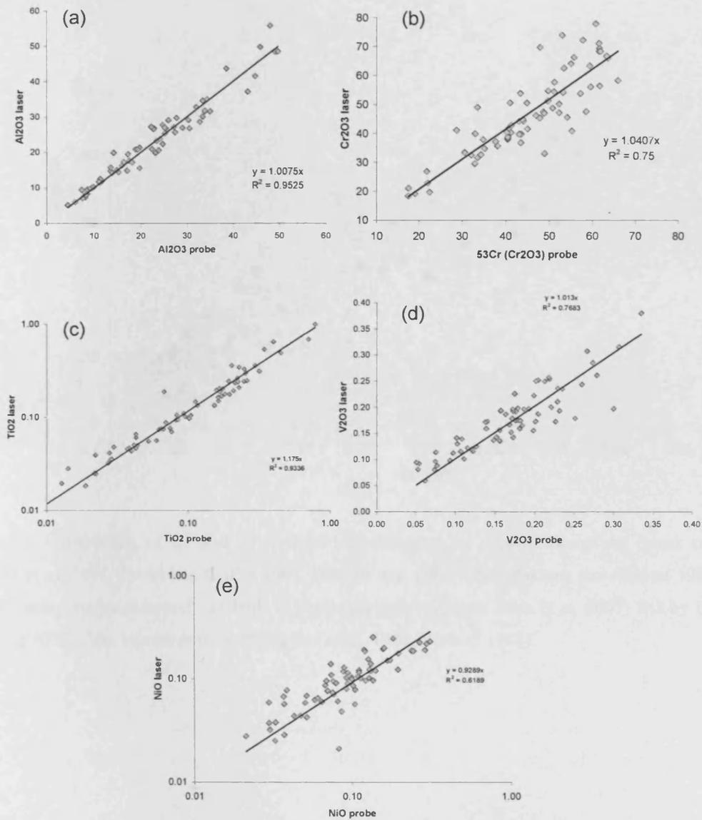
Figure 13: Comparison of laser-ablation ICP-MS and electron microprobe data for  $\text{Al}_2\text{O}_3$  (a),  $\text{Cr}_2\text{O}_3$  (b),  $\text{TiO}_2$  (d),  $\text{V}_2\text{O}_3$  (e) and  $\text{NiO}$  (f).  $R^2$  = correlation coefficient.
