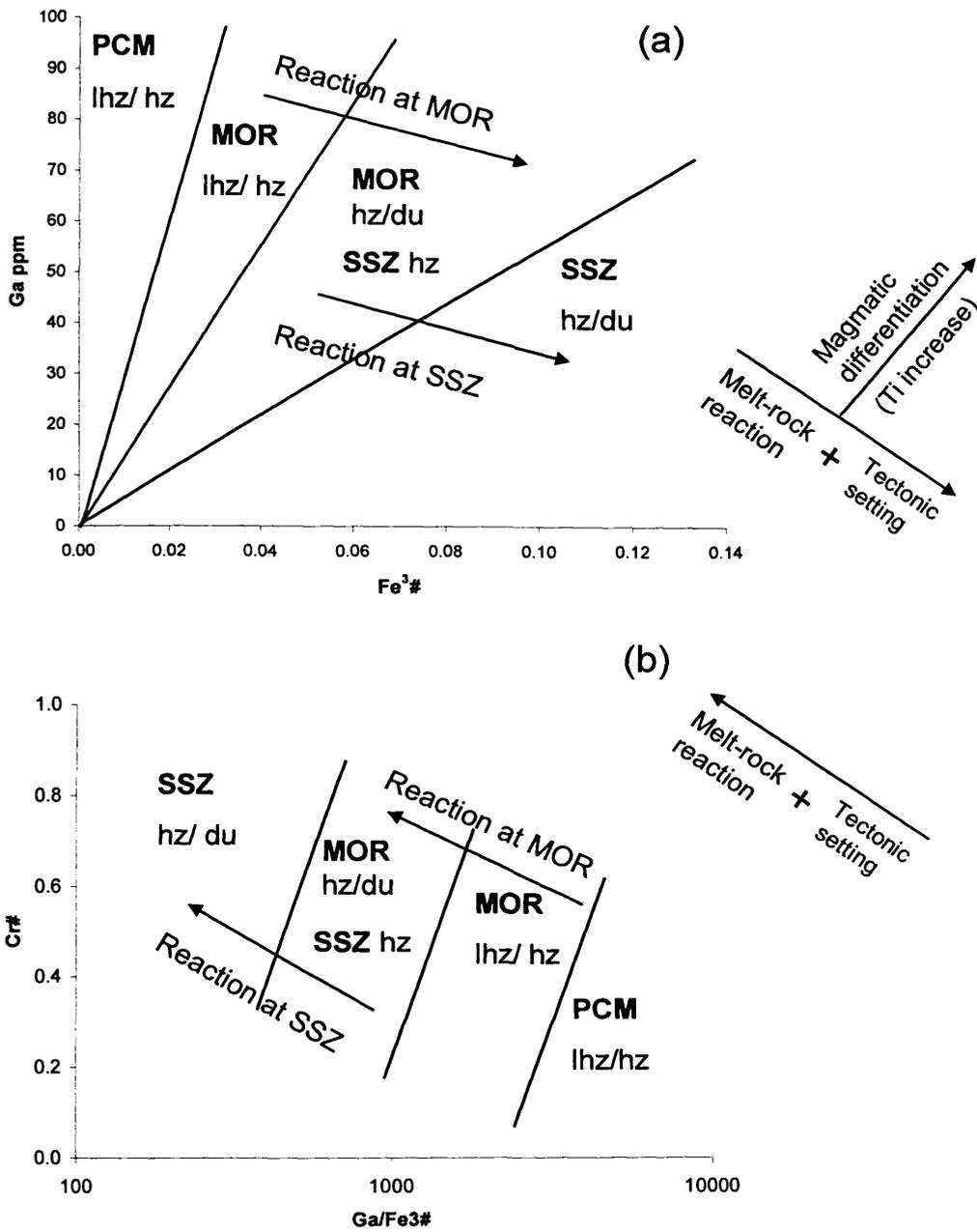
Figure 5.12: Finalised diagrams for (a) Ga vs.  $Fe^{3\#}$  and (b) Cr# vs. Ga/ $Fe^{3\#}$  which discriminate peridotites into four fields: PCM residual lhz/hz, MOR lhz/hz, SSZ hz/du and an overlapping field for MOR hz/du and SSZ hz. Vectors are marked schematically for tectonic setting, melt-rock reaction and magmatic differentiation. They show that Ga/ $Fe^{3\#}$  ratios are independent of magmatic differentiation but dependent on both tectonic setting and melt-rock reaction.
