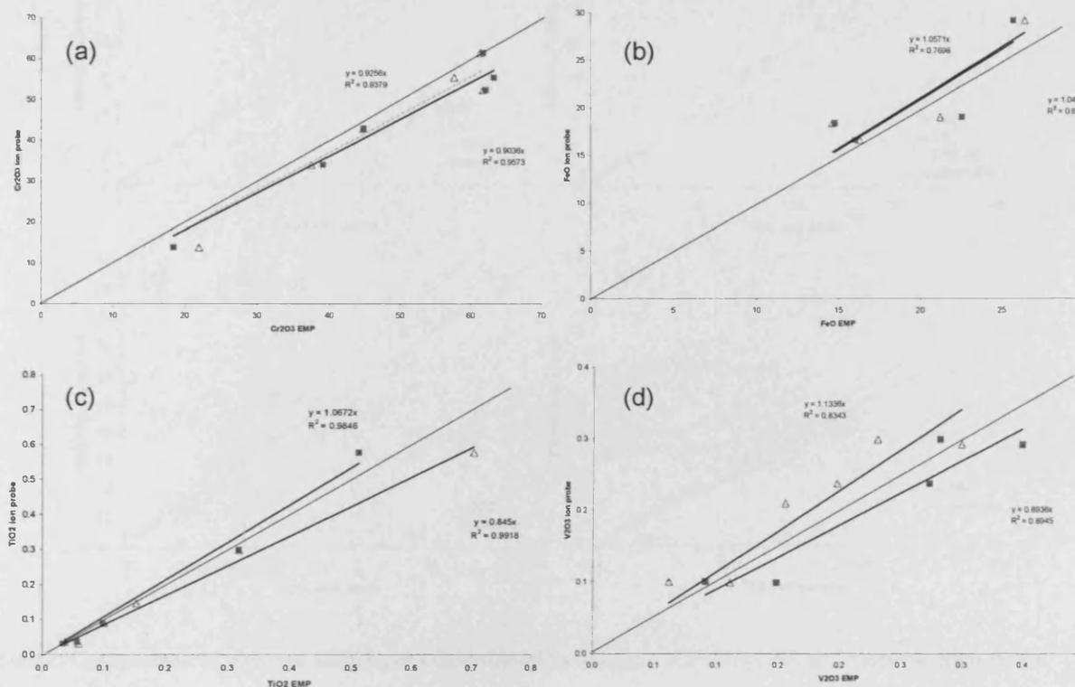
Figure 1: Comparison of element abundances determined by electron microprobe (triangle analysed by SD, square analysed by JAP) and ion probe for (a) Cr<sub>2</sub>O<sub>3</sub>, (b) FeO, (c) TiO<sub>2</sub> and (d) V<sub>2</sub>O<sub>5</sub>. Solid line marks 1:1 correlation line.
