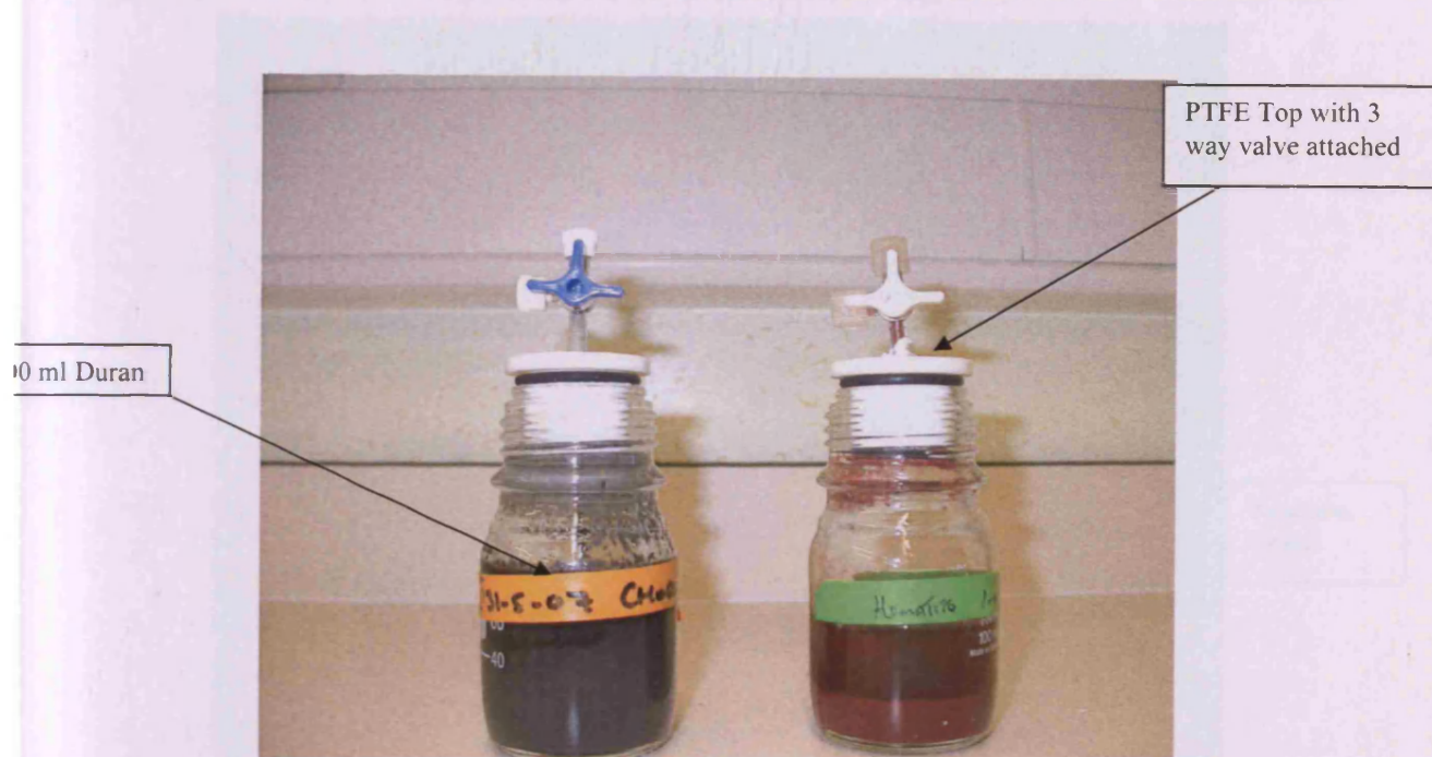
Fig 2.6. Type 3 reaction vessel (PTFE stopperd duram bottle)
