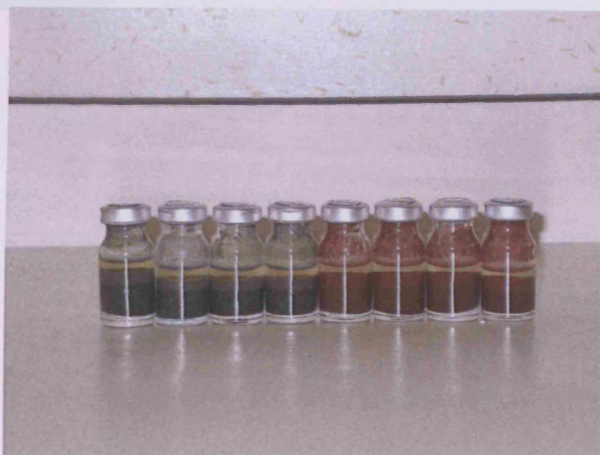
Fig 2.7. Type 4 reaction vessel Wheaton® serum vials
