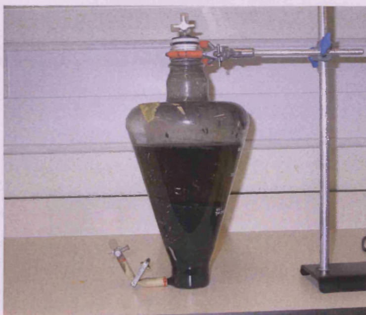
Fig 2.5. Type 2 reaction vessel (inverted modified conical flask)
