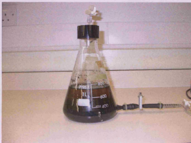
Fig 2.4. Type 1 reaction vessel (modified conical flask)
