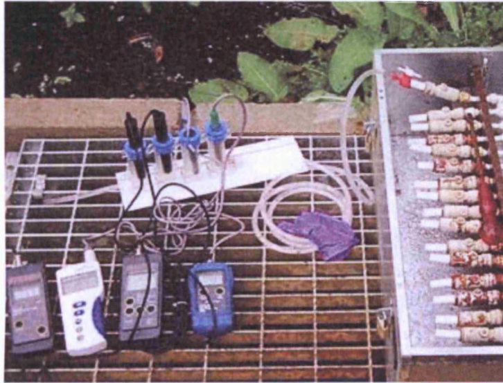
Figure 5-2: VFR sample port monitoring using a Watterra Sheffield flow through cell and hand held meters
