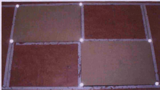
Figure 4.35 Calibration panels positioned on top of each force plate
