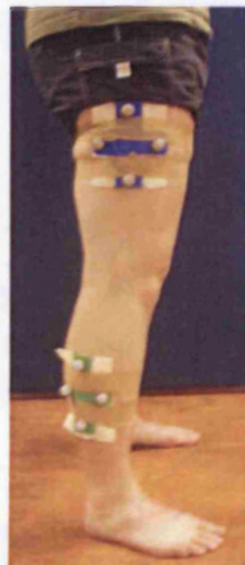
Figure 2.5 Marker clusters positioned laterally on the shank and thigh and secured using Coban TM tape
