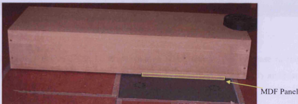
Figure 4.2 MDF Panel providing Interface between step 1 and a force plate
