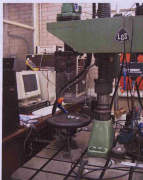
Figure 4.9 Calibration of a cylindrical weight using a load cell
