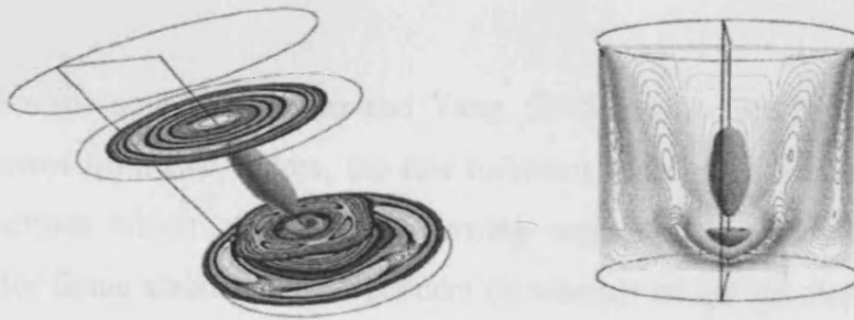
Figure 2.1. Vortex breakdown seen from different angles (Serre and Bontoux, 2002)
