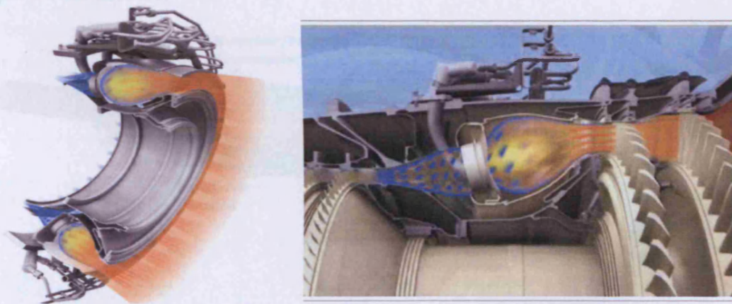
Figure 1.11. Combustion systems in to a gas turbine (GE Aviation, 2006)
