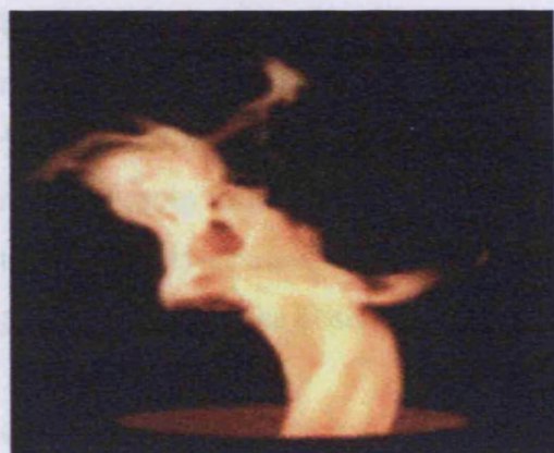
Figure 2.5. Visualization of the helical nature of a single PVC (Syred, 2006; Fick, 1998)
