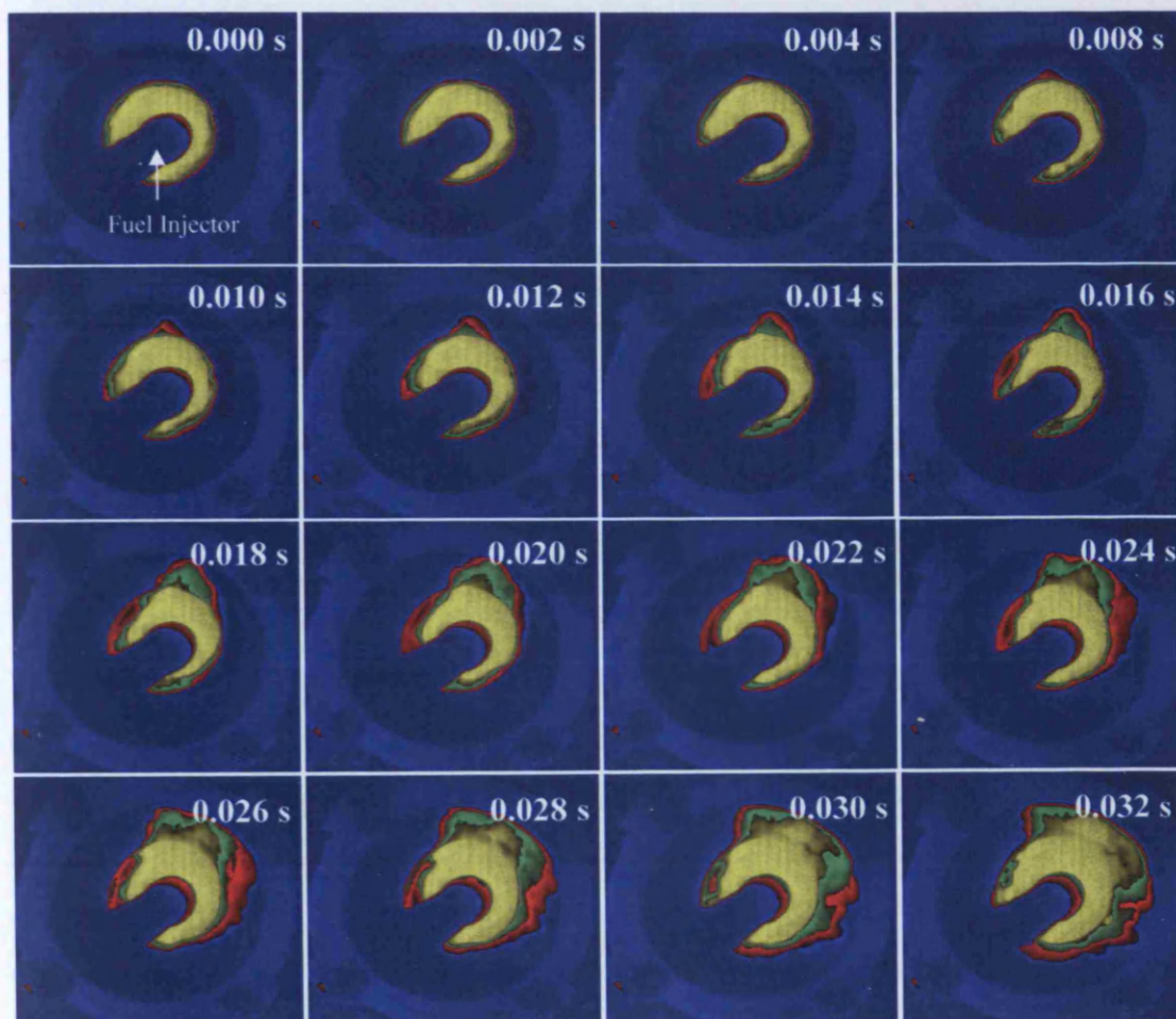
Figure 6.20. First moments of propagation. The flame moves practically radially, with slower motion in the tangential direction. Air flow injection of 600 l/min, 0.60 l/mi gas (100% Premixed injection, \phi = 0.95 ). The intensity scale as in figure 6.13.
