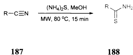
Scheme 93. Facile methods for synthesis of primary thioamides under MW irradiation at 80 °C.
