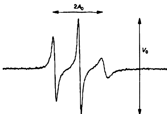
Figure 2.10; EPR spectrum of 16-DSE in 25mM SDS solution
