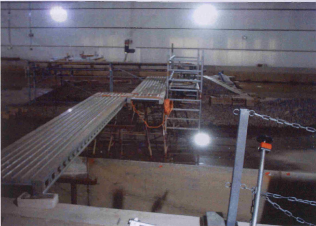
Figure A1- 11. The walkway that connected the model beach with the side of the wave basin
