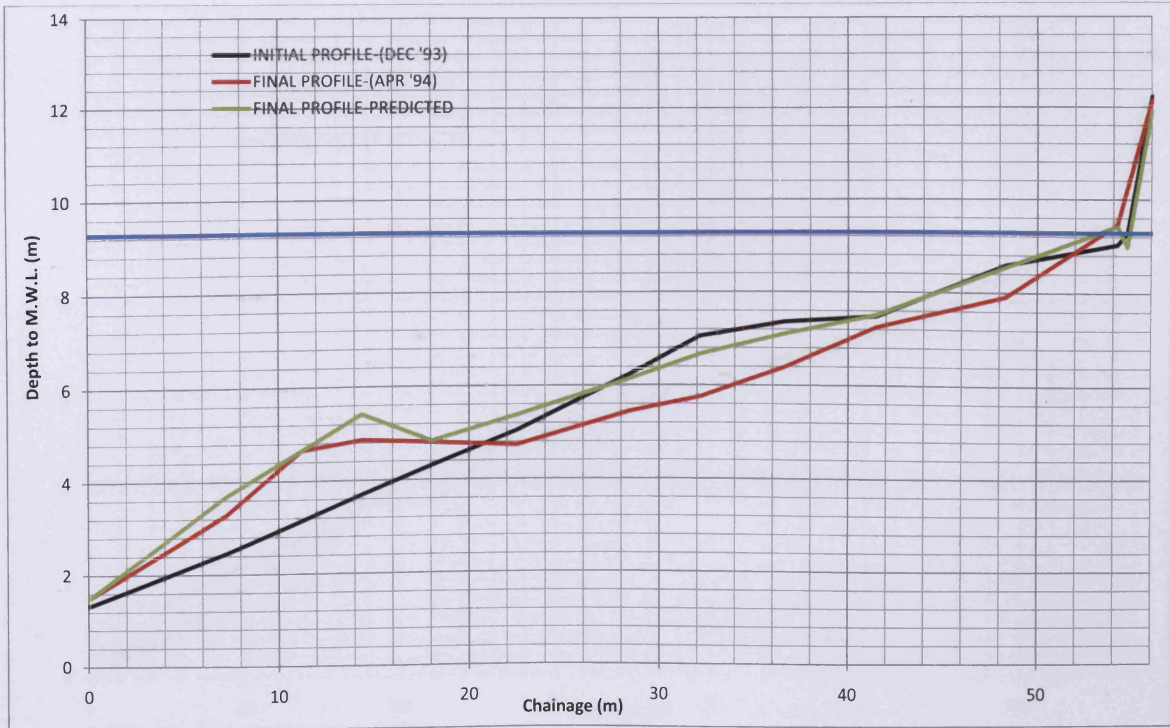
Figure A4- 5 Comparison of predicted and measured beach profile for location A-North (December '93-April '94)
