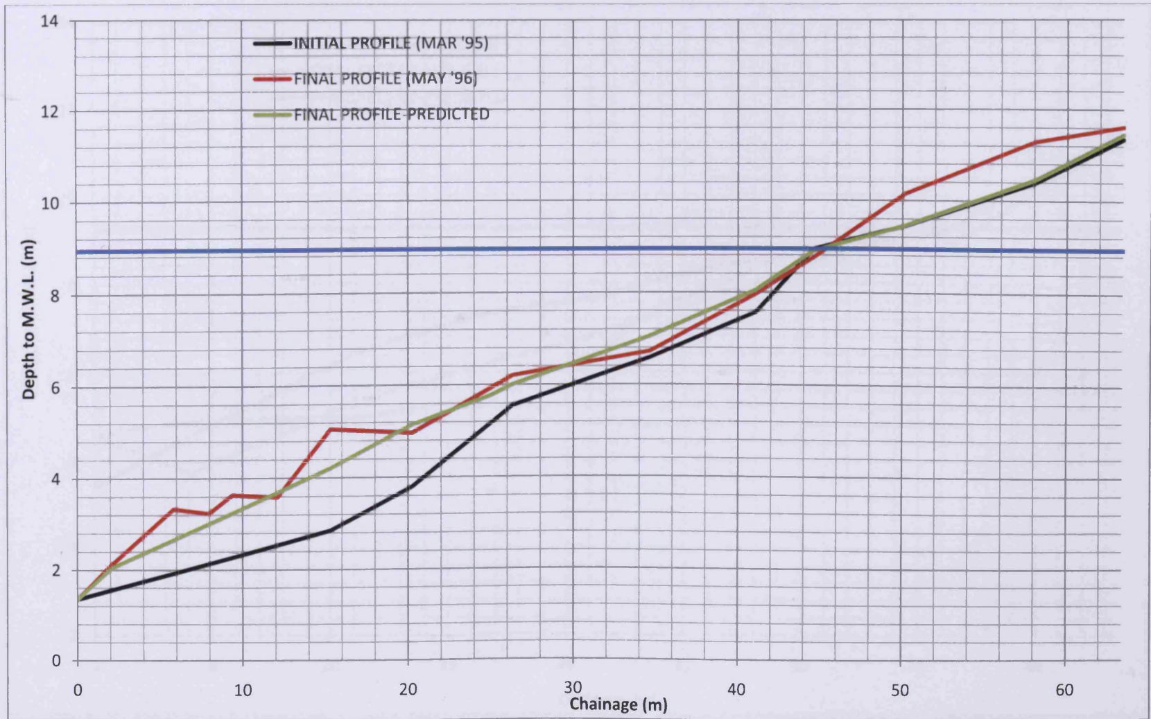
Figure A4- 20 Comparison of predicted and measured beach profile for location B-North (March '95-May '96)
