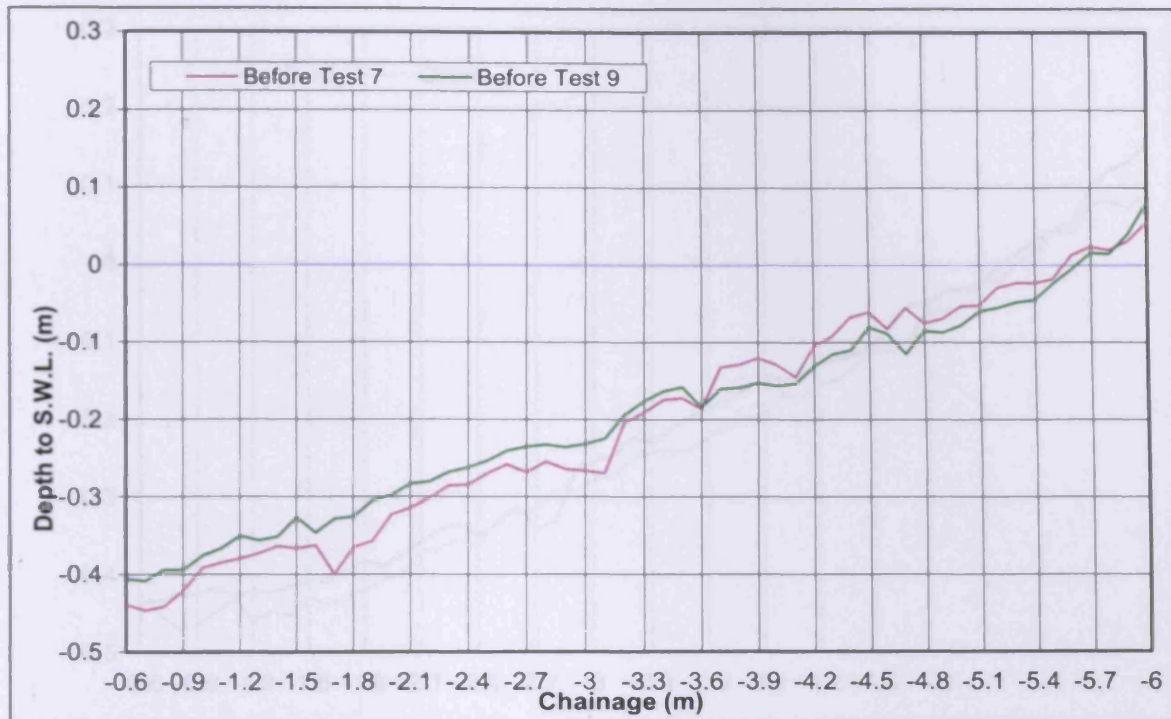
Figure 4-52 Original cross-shore profiles of Line 3 (Mixed Beach)
