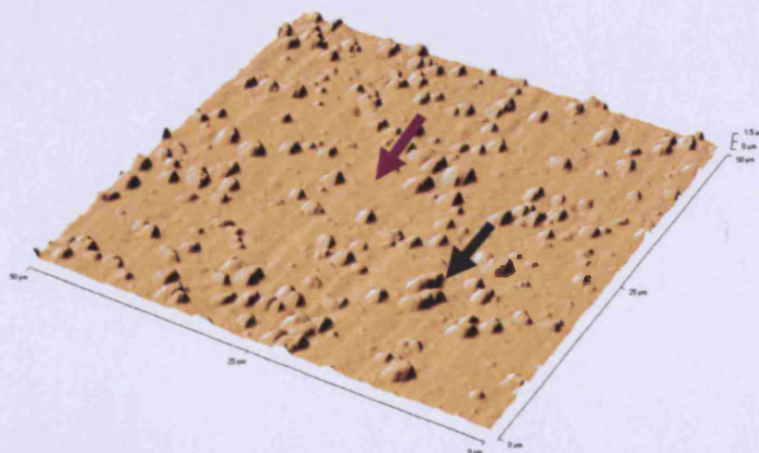
Figure 2.7. AFM of TAN samples. Protruding micro-spiked structures appearing pyramidal (Blue arrow) observed in the positive control (A), are eliminated by electropolishing (B). The remnants of these structures are observed embedded within the material (White arrow). In contrast paste polishing (C) appears to produce a smooth base material (Purple arrow) but fails to remove the protrusions although it does appear to have extensively reduced them (Black arrow) compared to the positive control.
