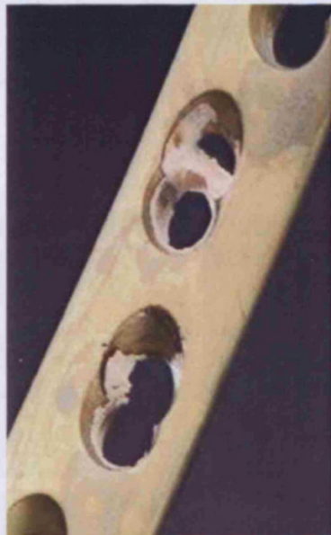
Figure 5.1. Bony in-growth to the plate hole of a LCP after implantation within a sheep during experimental study. Picture courtesy of the AO Research Institute.
