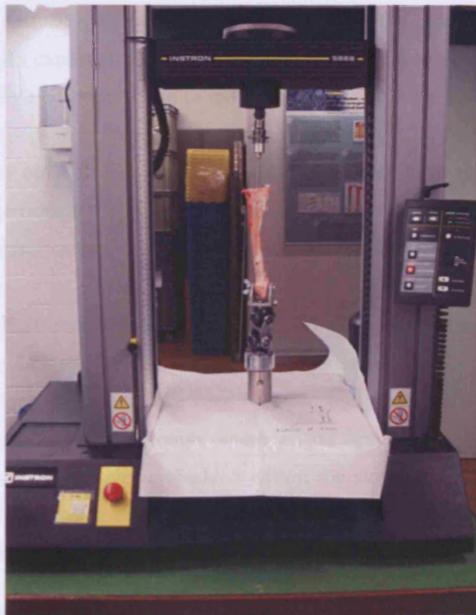
Figure. 6.1 Testing Device, with adapter screwed into the endcap holder of the nail within the tibia before pull out was performed. A constant force of 1mm/min was applied.
