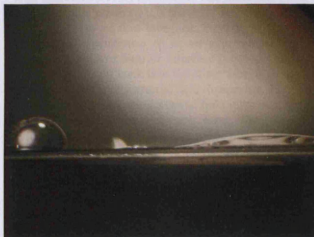
Fig. 3. Contact angle of the hydrophobic silver and hydrophilic borosilicate glass.
