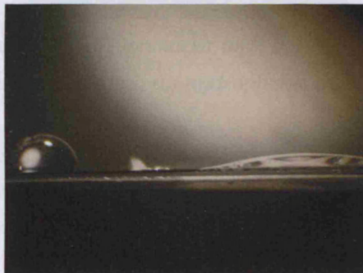
Figure 6 – 6: Contact angle of the hydrophobic silver and hydrophilic borosilicate glass
