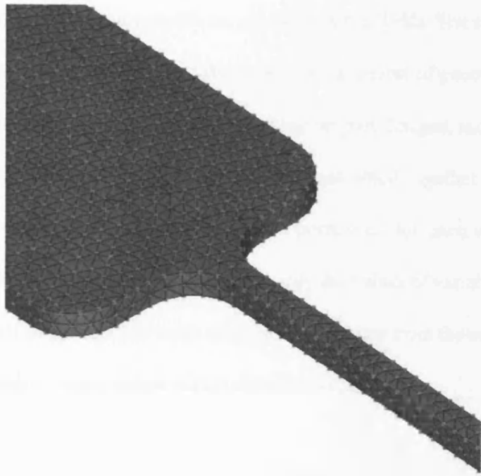
Figure 5.1 The CAD model meshed employing the hybrid FEM-FDM approach
