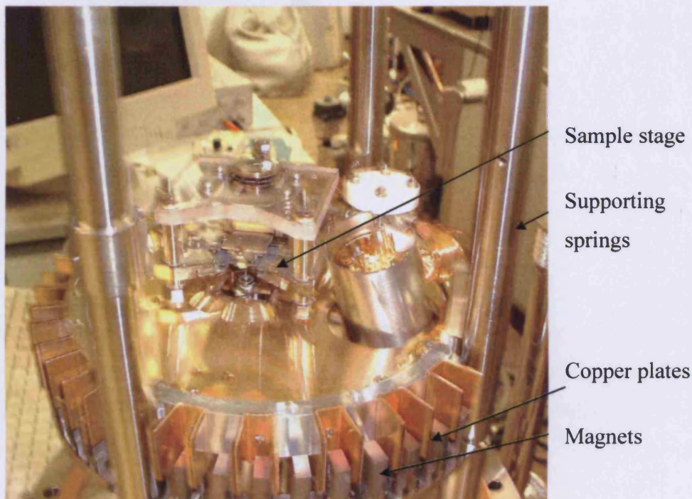
Fig. 3.4: Vibration dampening instrumentation.
