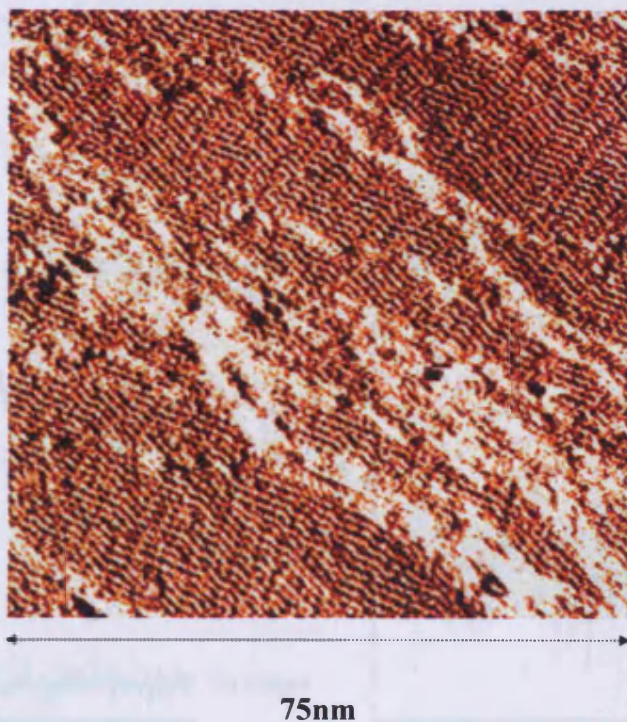
Fig.5.6: 'zig-zag' structure at the surface after exposing a partially oxidised surface to 100L of aniline.
