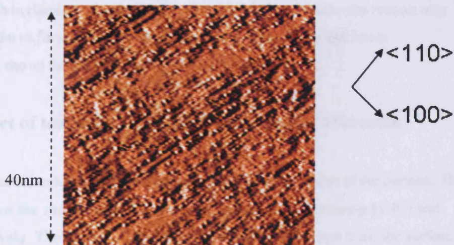
Fig. 7.4 STM image after a dose of 300 seconds of melamine at a Cu(110) surface at 290K [bias: negative, voltage = 0.99V, current = 3.32nA].
