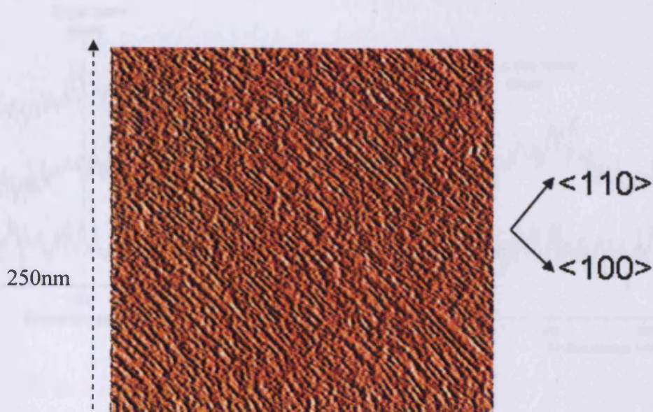
Fig. 9 STM image after a dose of 180 seconds of melamine at a fully oxidised Cu(110) surface at 290K [bias: negative, voltage = 1.33V, current = 1.87nA].
