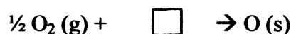
Figure 5.3 – Proposed reaction scheme for the oxidative dehydrogenation of propane 3 . (g) is gaseous substrate and product, (s) is adsorbate on the surface, \square is an oxygen vacancy.
