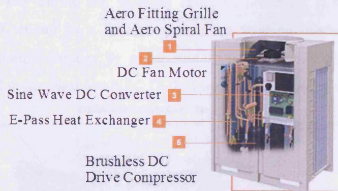
Fig. 1-11 Brushless PM DC Drive compressor with a Daikin Variable Refrigerant Volume (VRV) System [1-48]
