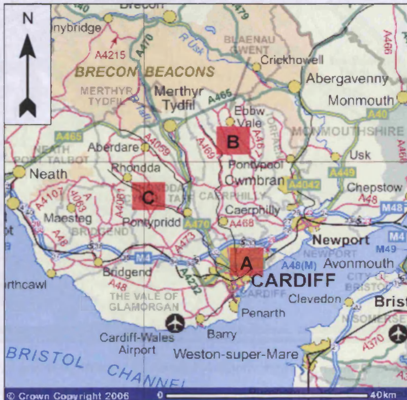
Figure 1.17: Landfill sites of interest in south Wales. Adapted from OS Miniscale™ series. Landfill A = active and partially lined site; Landfill B = active, dilute and disperse site; Landfill C = inactive restored and contained site.
