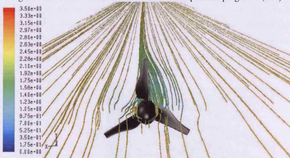
Figure 9.16: Disrupted downstream vortices with upstream profiled flow (m/s)
