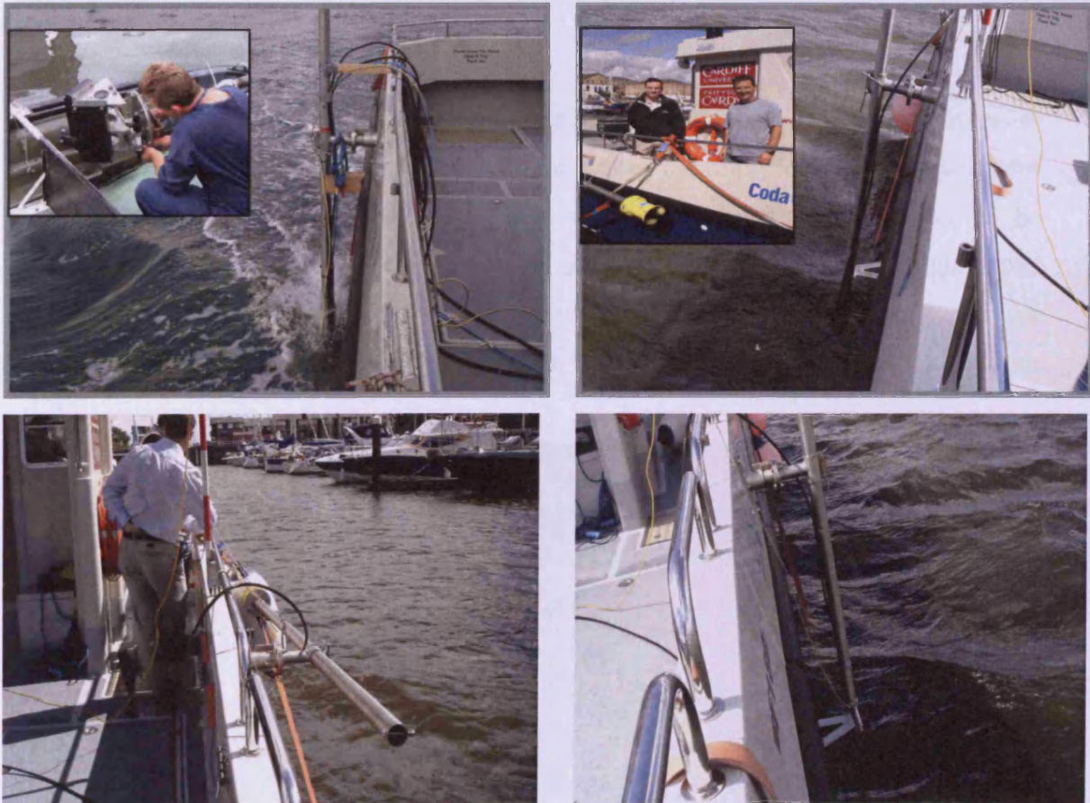
Figure 5.10: ADCP and bathymetric survey aboard the CodaOctopus Guiding Light
