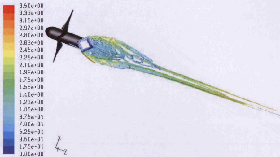
Figure 9.24: Plan view of Pathlines coloured by velocity magnitude with diamond cross section
