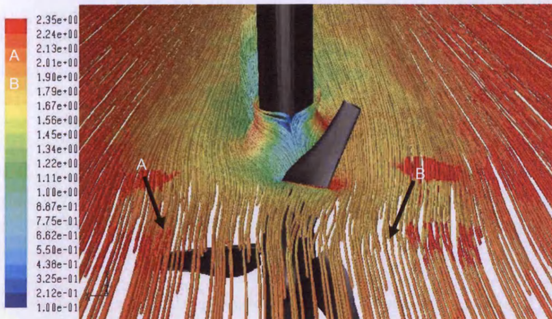
Figure 9.40: Pathlines coloured by velocity magnitude (m/s) with downstream stanchion
