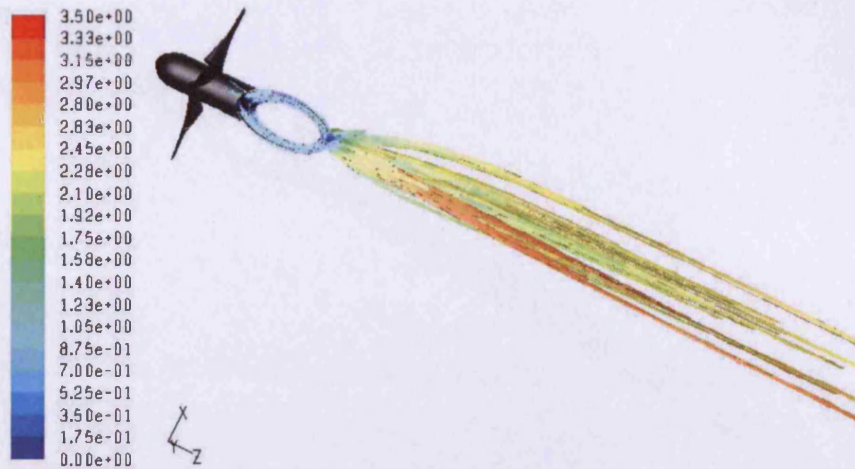
Figure 9.18: Plan view of Pathlines coloured by velocity magnitude with elliptic cross section
