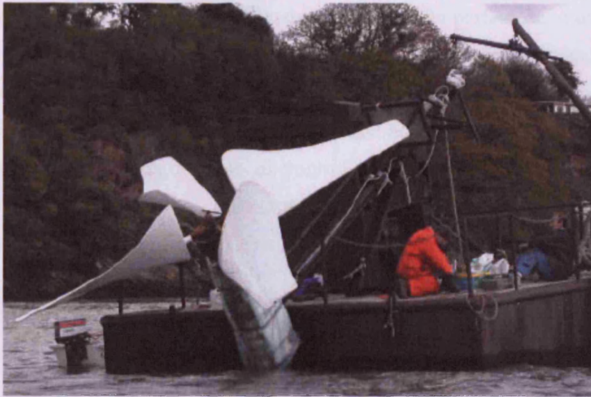
Figure 2.14: River trials for a 4 bladed 5.5m turbine with a flow speed of 0.9 m/s Source: Egarr et al, 2004
