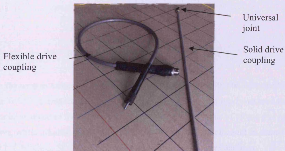
Figure 5.5: Flexible and solid drive shaft couplings
