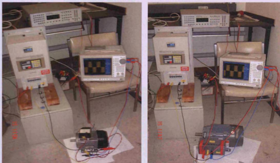
Fig. 6.6. Experimental set-up with TOSHIBA VF-A3 inverter
