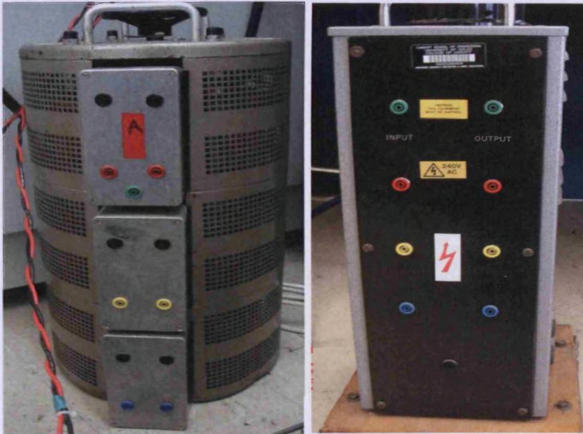
Fig. 4.10. Three-phase variable transformers A and B
