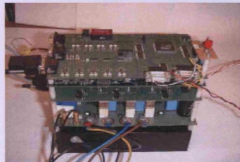
Fig 2. Three-phase 7.5kW matrix converter
