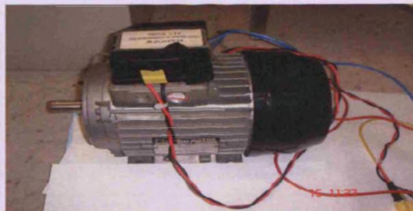
Motor B is an induction motor of nominal power 2.2 kW. Its main parameters are introduced in table 6.2. Resistance and inductance of stator windings were measured by the multimeter and impedance meter used for motor A (§ 4.2.2).
