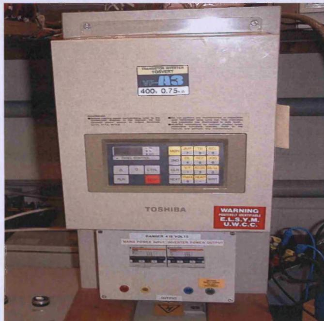
Fig. 4.4. DC-link indirect converter [TOSHIBA –TOSVERT VF-A3]
