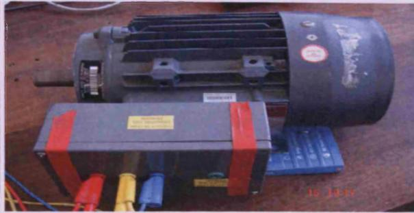
Both motors were supplied under sinusoidal voltage (50 Hz) via variable transformer A (§4.2.2) at an RMS line-line voltage  $U_{lock}$  of 200V. The shaft of the two induction motors was locked while the RMS current  $I_{lock}$  [A] was measured by the multimeter (§.4.2.2). The rotor impedance  $|Z_2'|$  [ $\Omega$ ] is calculated based on experimental measurements as the product of stator impedance  $|Z_1|$  and a factor  $\kappa$ .
