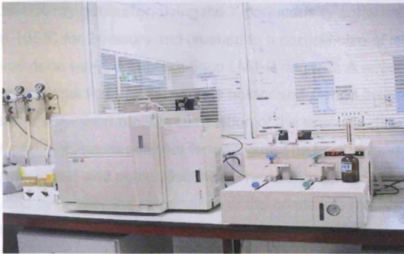
Figure 6.10 SHIMADZU analyser in use for inorganic carbon analysis
