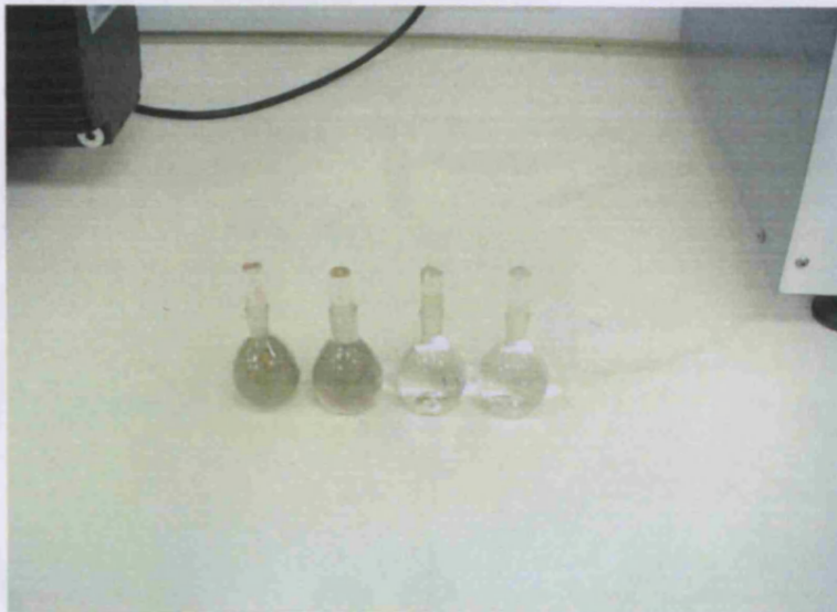
Figure 6.7 Measuring bulk density using a pycnometer
