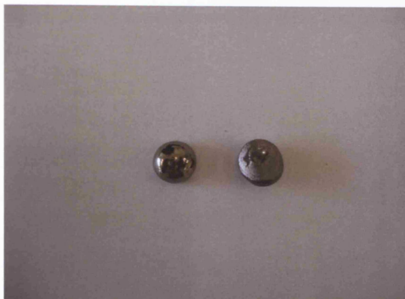
Fig. A1.3 Gd 5 Si 1.8 Ge 2.2 and Gd 5 Si 1.9 Ge 2 samples prepared by arc-melting before cutting at The University of Birmingham.
