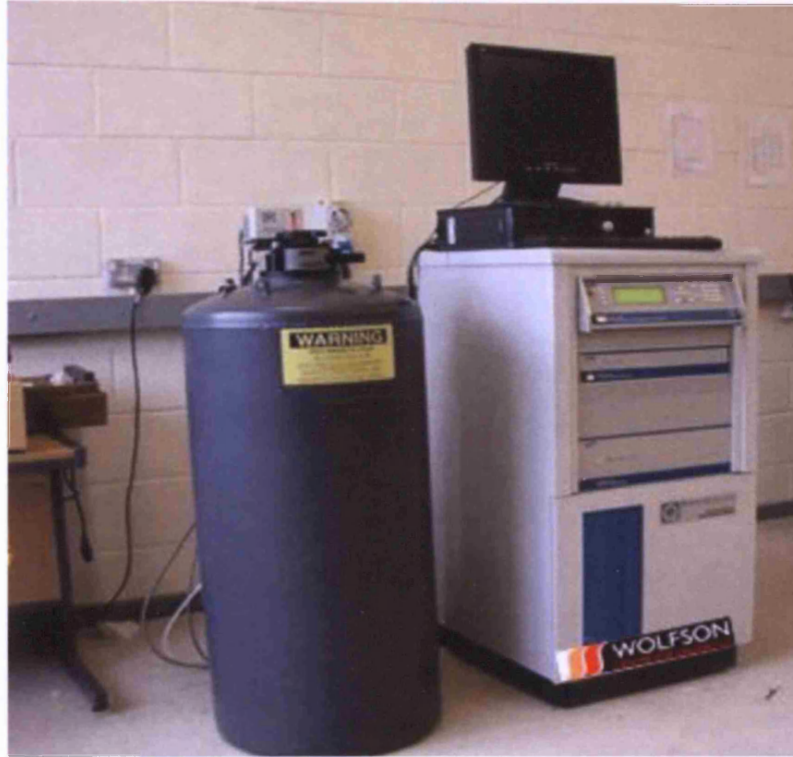
Fig. 5.5 Physical Properties Measurement System (PPMS) at Wolfson Centre. Cryostat contains a sample chamber which controls temperature, pressure and magnetic field.
