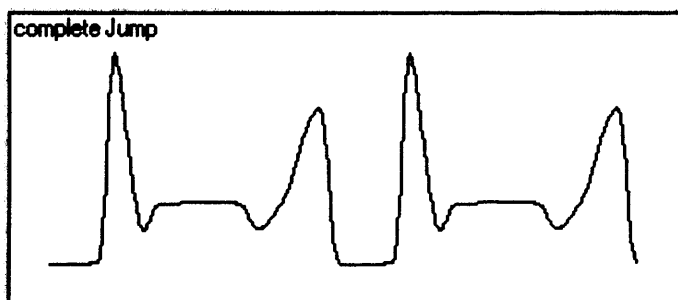
Fig. 1.7: Loading pattern of the complete jump waveform applied during daily loading onto cancellous bone explants cultured in the ZetOs system.
