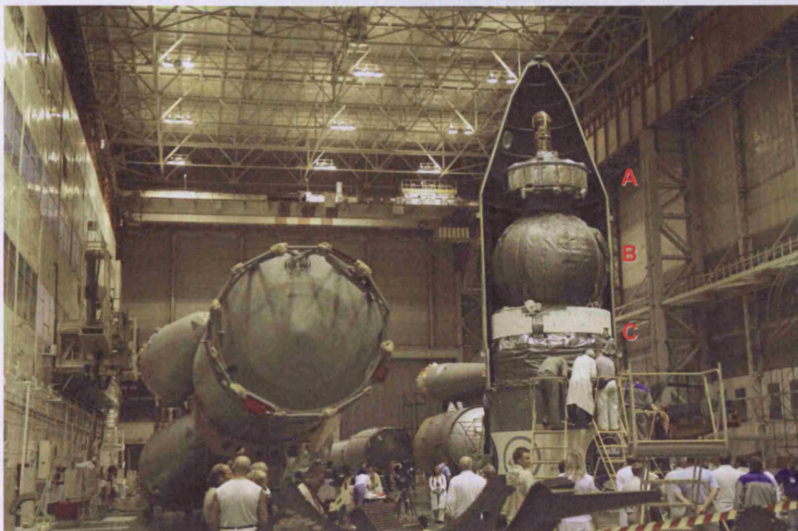
Fig. 3.1: Image of the Foton spacecraft (right side) inside and next to the Soyuz-U launcher unit prior to launch. The Foton consisted of 3 modules – the battery module which provided the payload with 500 W daily (A), the re-entry module that housed the scientific payload (B) and the service module that contained the attitude control system (C). Image source www.esa.int .
