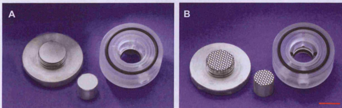
Fig. 4.13: Images show culture chambers for the ZetOs system. A: Normal culture chamber with smooth baseplate and piston surface. B: Honeycomb-surfaced chamber design with applied 0.2 mm deep channels on baseplate and piston surface. Scale bar represents 1 cm.
