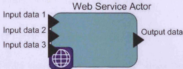
Figure 2.4: A Kepler actor with multiple inputs.
