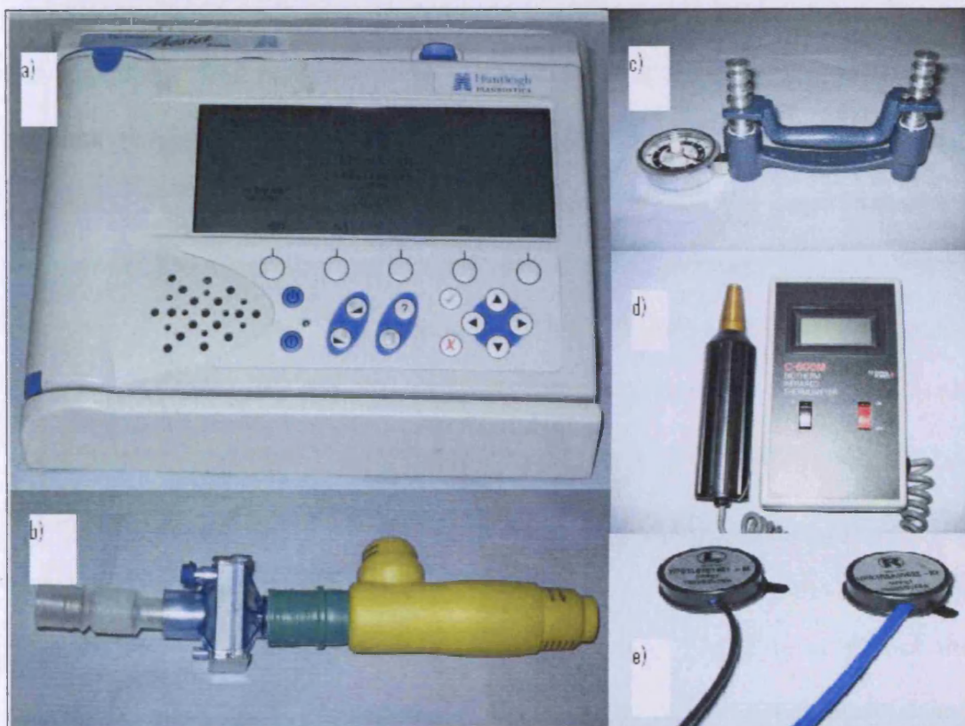
Figure 4.3: a) Huntleigh Vascular Assist®; b) PowerLung® BreatheAir® c) Baseline® Hydraulic Hand Dynamometer; d) IR temperature sensor and e) PPG probes
