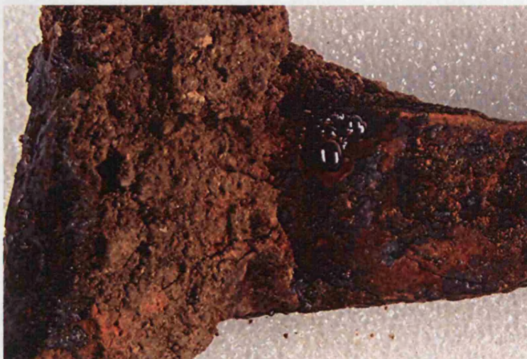
Figure 2: Archaeological iron nail showing a bubble-like structure formed during exposure of the object to 75% RH. The bubble is 2 mm across and probably composed of akaganéite.
