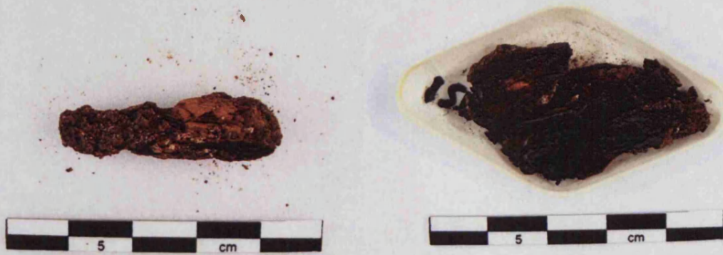
Figure 40: BOR_6151 before (left) and after (right) accelerated corrosion testing. This untreated object was completely fragmented during the test.
