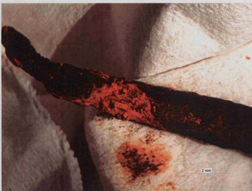
Figure 69: Rinsing nail 2, showing development of orange corrosion on the surface after rinsing. The product was very powdery and non-adherent and identified as lepidocrocite.
