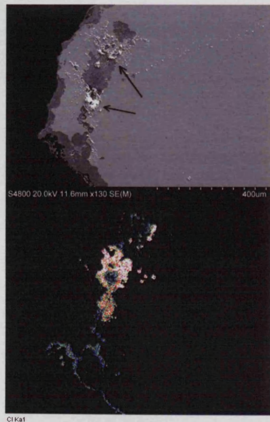
Figure 31: BOR_1693.2. SEM image (top) showing fresh corrosion on the polished surface located near cracks in the corrosion structure (arrowed). The EDX map (bottom) shows high levels of Cl in these areas. Cl is also located on the metal/corrosion interface and along the outer edge of the sample.
