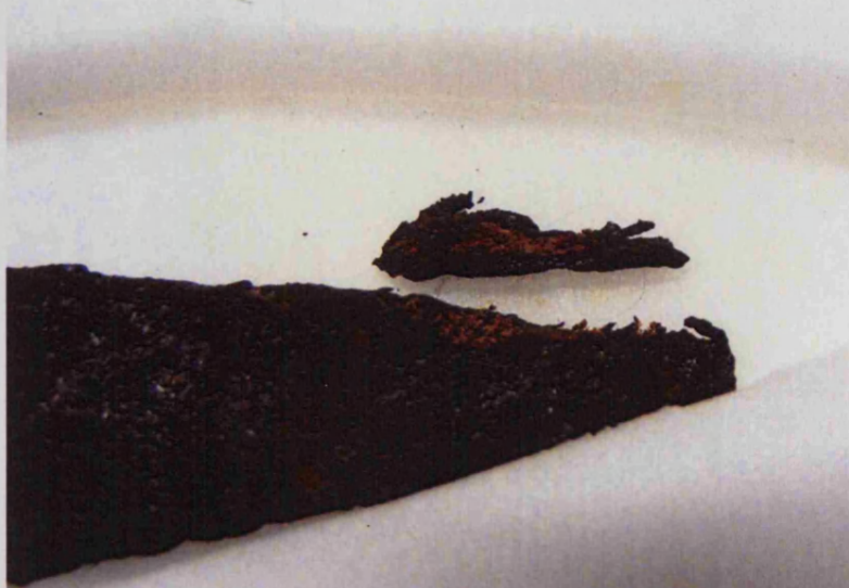
Figure 3: The tip of an Anglo-Saxon spearhead where the formation of akaganéite crystals has resulted in a large flake of the corrosion layers being detached.
