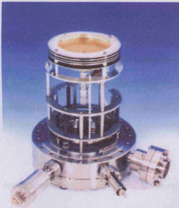
Figure 2.7. Omicron SpectralLEED system. The grids are clearly visible at the top and the view-port is at the bottom. The magnetic shield has been removed.
