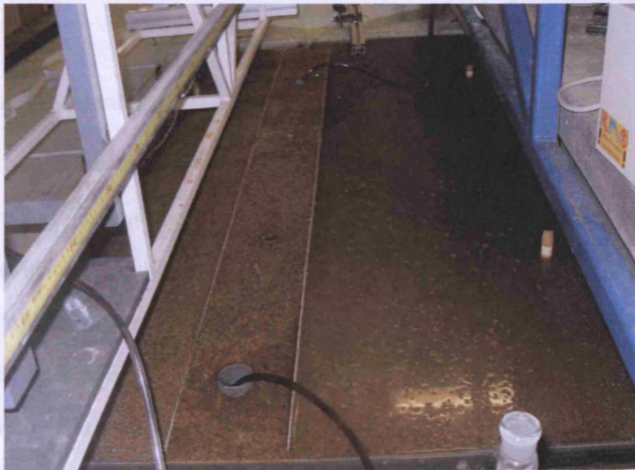
Figure 5.73: Tracer test in hole 4 with the pump in hole 1.
