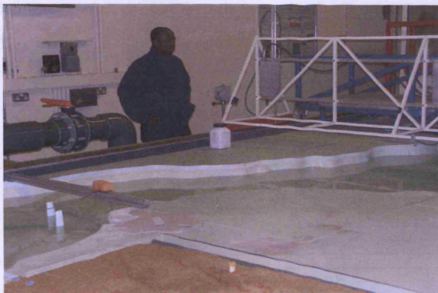
Figure 5.52: (a) Tidal basin showing water level and ADV probes and (b) water level probes for data collection
