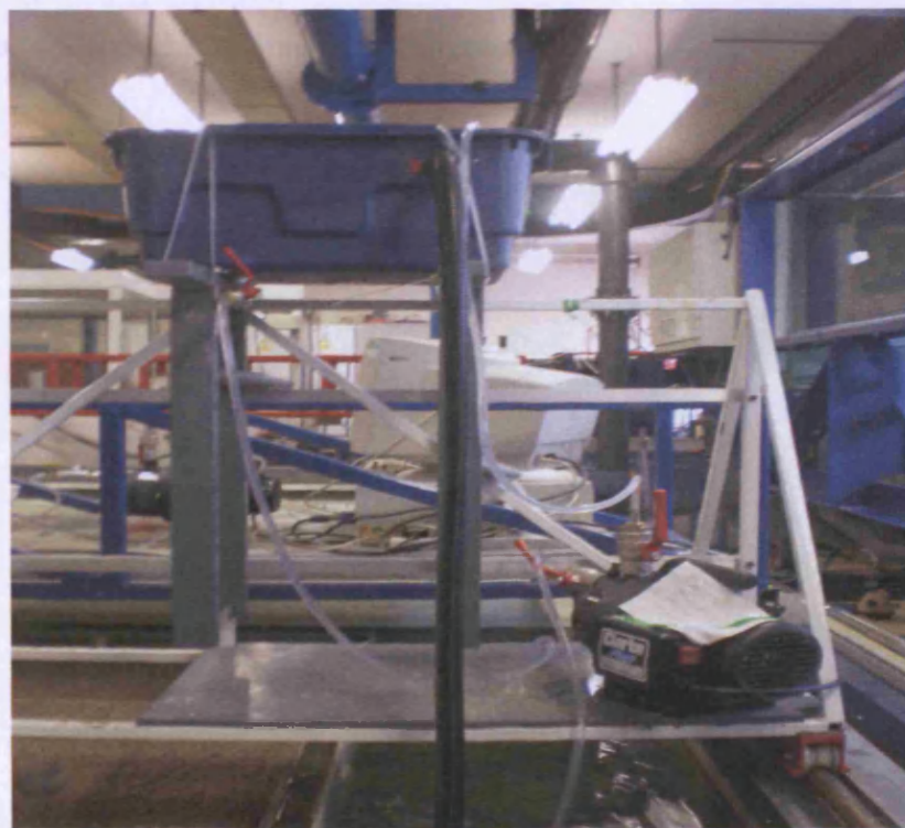
Figure 5.69: Experimental set up for water level measurement at the weir
