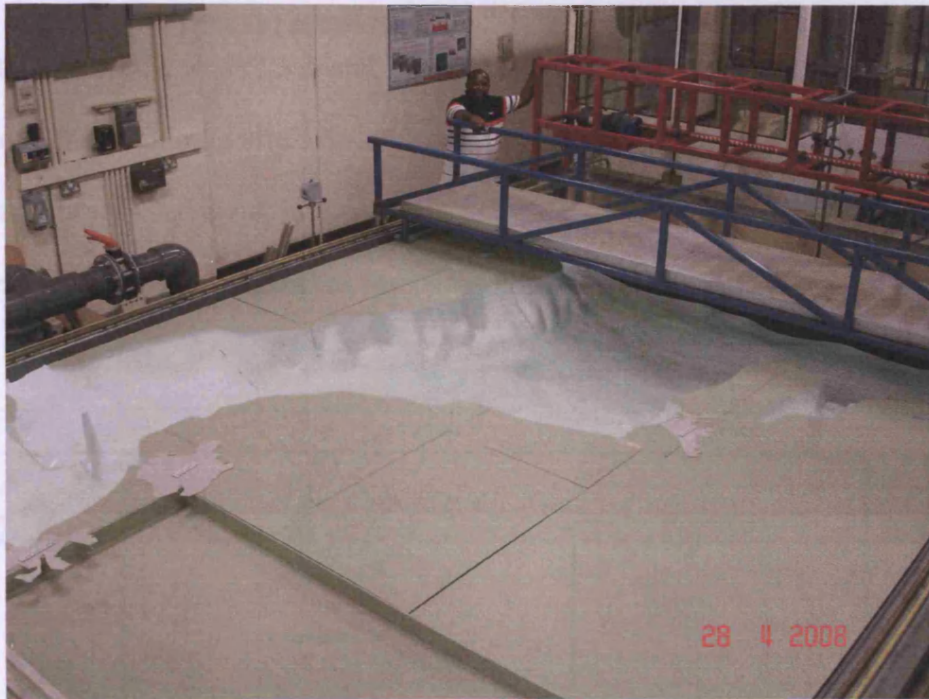
Figure 5.49: Side view of the physical model as laid out in the tidal basin
