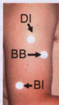
FIGURE 2.13: Modified Humerus Technical Coordinate System consisting of three markers placed on the insertion of the deltoid (DI), the biceps belly (BB), and the brachioradialis insertion (BI).
