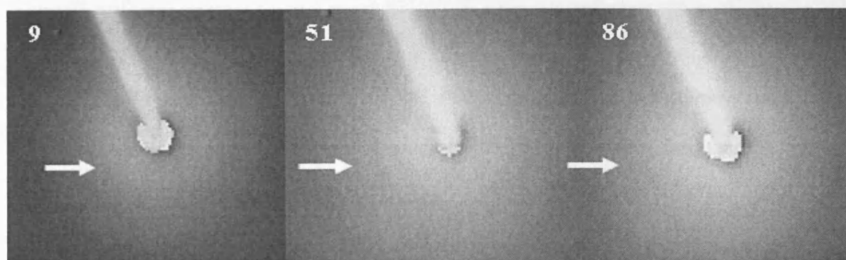
Figure 7.11: Three representative two-dimensional diffraction images from sample GD202r. The images correspond to scan numbers 9, 51 and 86. The presence of collagen axial diffraction is highlighted on each image by the presence of a white arrow.
