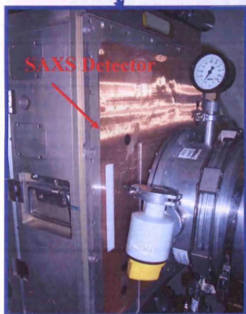
Figure 3.7: Image of station 2.1 at SRS Daresbury, with a sample to detector distance of 5.5m. The detector and sample areas are shown in detail in two additional images below the main image. The black dashed arrow indicates the direction of the incoming X-ray beam.
