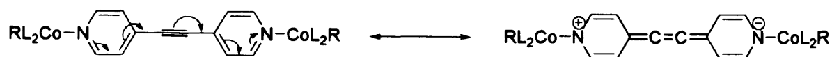
Scheme 5.12. Resonance forms of the BPA ligand, demonstrating the conjugation between the two pyridine rings.
