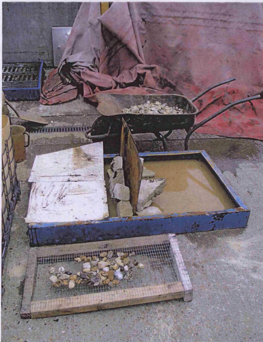
Figure 31: Split tank for shingle washing
