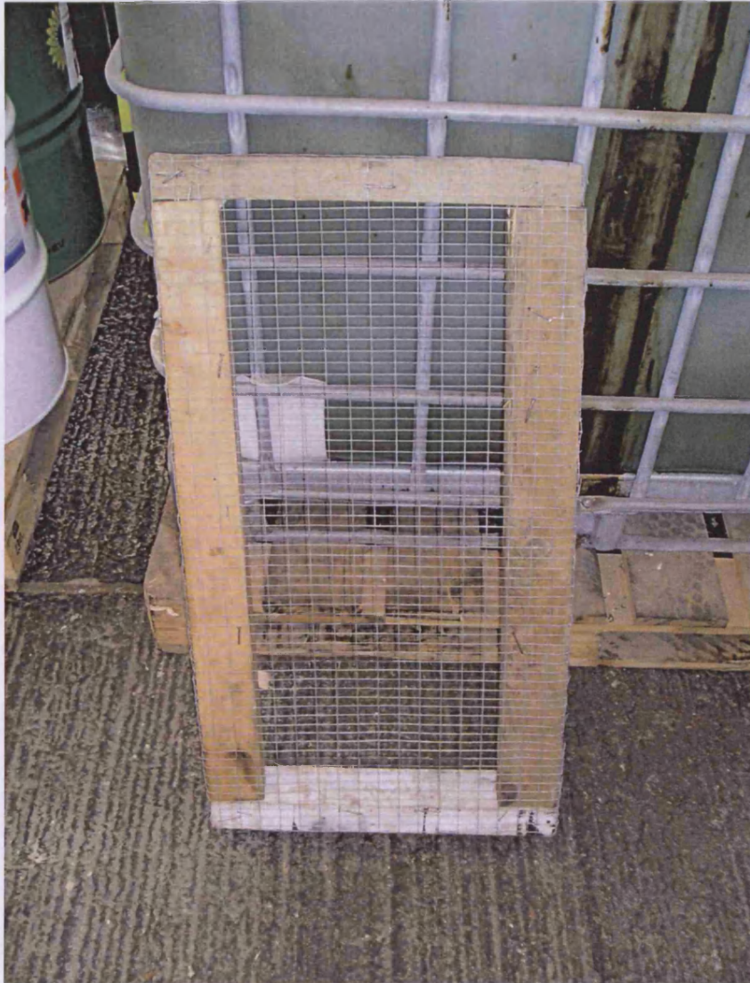
Figure 30: Mesh grid for aggravation of shingle samples
