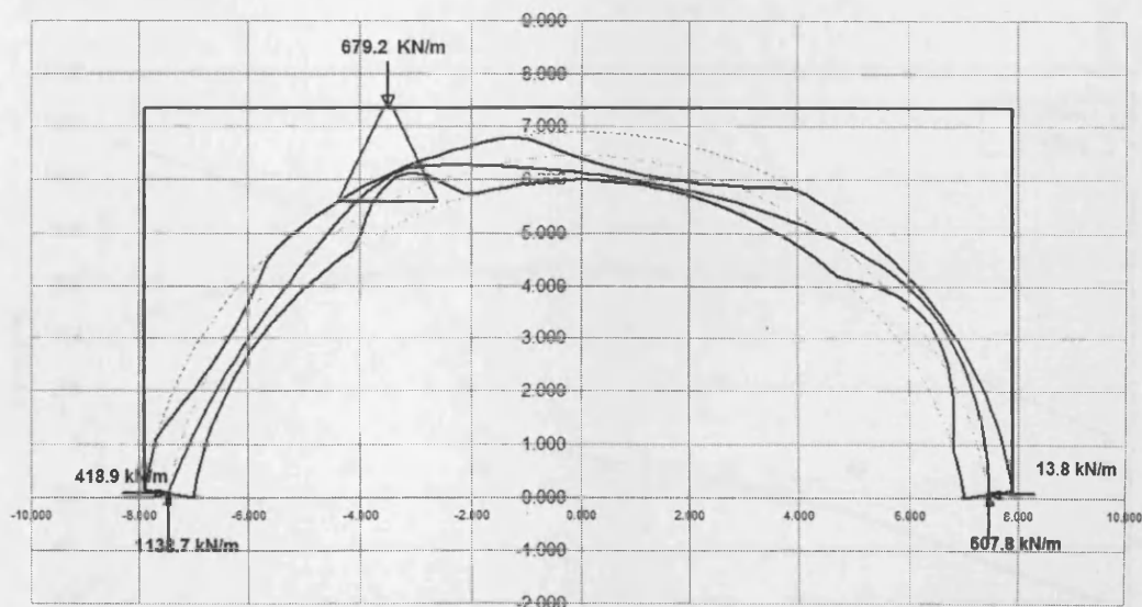
Figure 4.33 Arch view of quarter point ultimate load result
