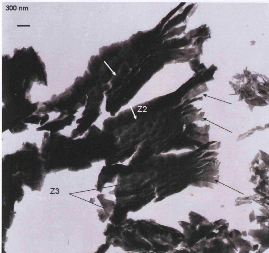
Fig.7.1: A transmission electron micrograph of particles in the well embedded-resin section. Three large particles appear to have a similar structure. Each particle shows three clearly defined zones: a light zone (Z1) showing a layered or sheet-like structure (dark arrows); a darker zone (Z2) at the center displaying aligned 'chatter pits', probably resulting from the diamond knife cutting (white arrows); an intermediate zone (Z3) having a smooth surface structure.
