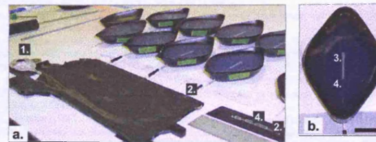
Fig. 9. (a) HF with directly coupled optical fiber LED excitation set up. (1) 650nm LED is the light source, the light is conducted through an (2) 1mm diameter optical fiber to the HF inside the phantom, providing direct illumination from one side of the HF. (b) Detail of the phantom made of 1% agarose gel in a black holder (~80x58mm at top widest points), the (3) HF is connected to the end of the optical fiber fitted with a (4) Tygon tube to help support the insert. Scale bar 20 mm.
