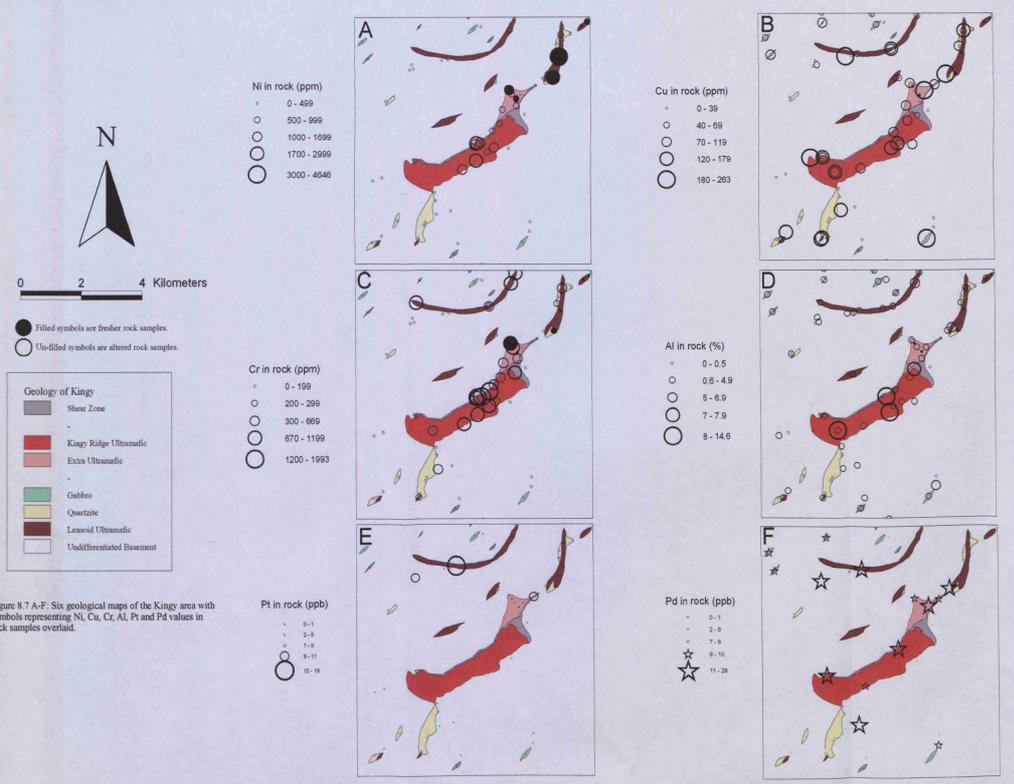
Figure 8.7 A-F: Six geological maps of the Kings area with symbols representing Ni, Cu, Cr, Al, Pt and Pd values in rock samples overlaid.
