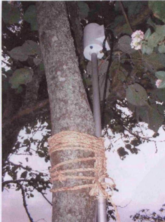
Figure 6.1: The magnetometer sensor set up aligned to N and attached to a tree.
