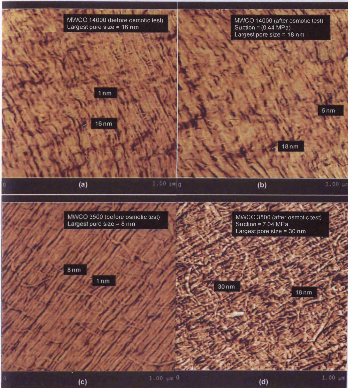
Fig. 6.7: AFM images of MWCO 14000 semipermeable membrane (a) before osmotic test; (b) after osmotic test; and images of MWCO 3500 semipermeable membrane (c) before osmotic test; (d) after osmotic test
