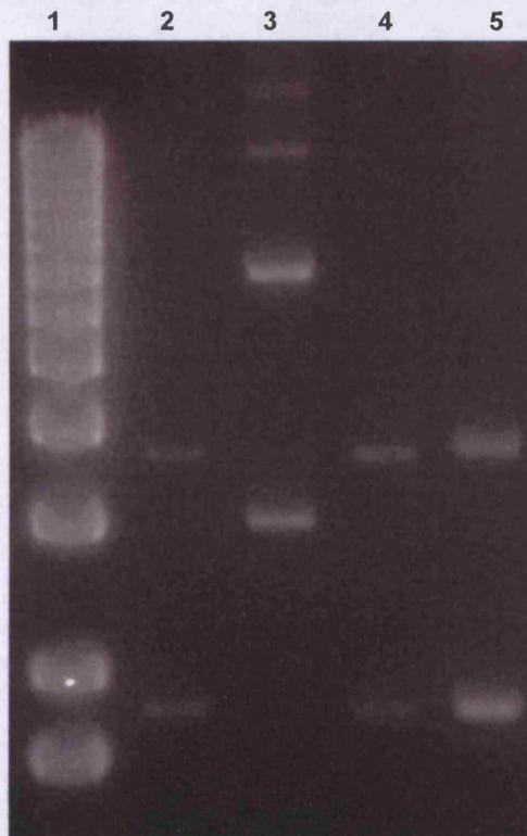
**Figure 3.3.6 Size screening for potentially positive colonies.** Plasmid DNA was isolated from potential 2Kbp 5'promoter/pGEM-T colonies using the alkaline lysis method as described in section 3.2.2.4.4. To identify potential positive colonies, plasmid DNA was separated by agarose (0.7 %) gel electrophoresis; lane 1, molecular weight markers; lanes 2, 4 and 5, show colonies with just the pGEM-T vector; lane 3, successful 2Kbp 5'promoter/pGEM-T colony.
