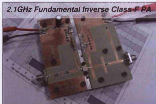
Fig. 4.19. Final high-efficiency prototype PA operating at 2.1GHz with measured output network insertion loss (right).
