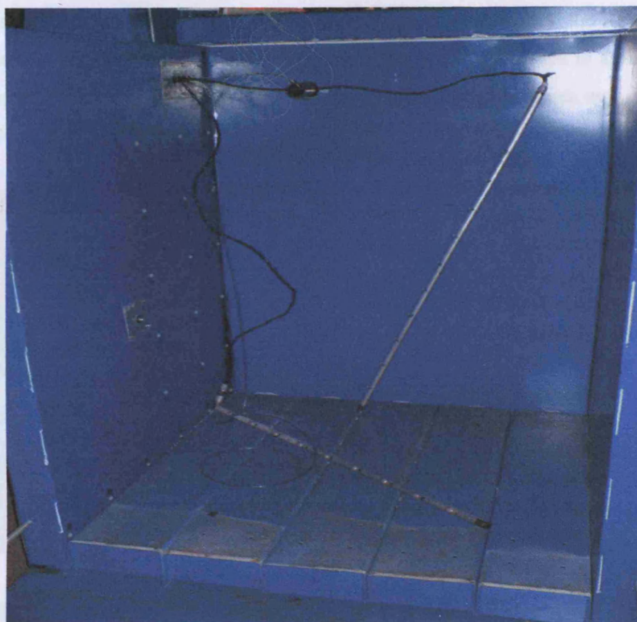
Figure 5.5 Compost side of test rig showing the 5 separate plenums and thermocouples mounted in the walls and probes.
