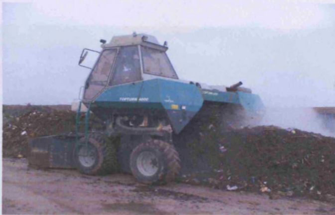
Figure 2.14. A self propelled windrow turner, turning a green waste windrow. This machine is capable turning a windrow 4 meters wide and 2 meters high.
