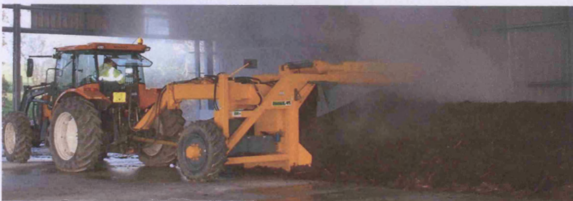
Figure 2.16. A tractor towed windrow turner. The turner is powered by the tractor engine and is capable of turning a windrow 4 meters wide and 2 meters high.
