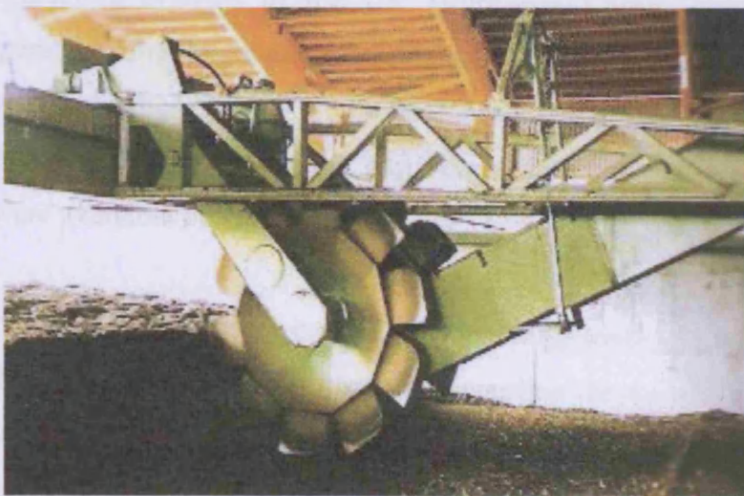
Figure 2.22. An image of the specialised equipment used in enclosed halls to turn and move waste through an enclosed hall composting system. (Composting Association, 2004).
