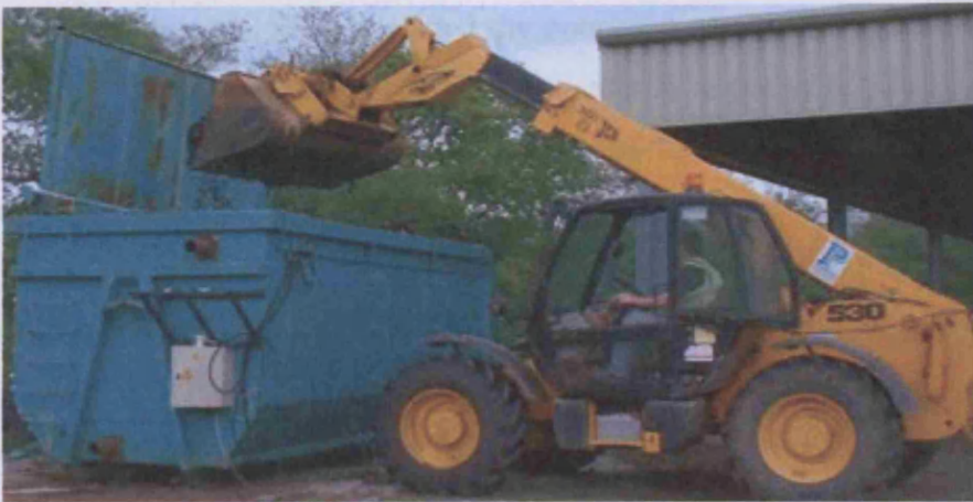
Figure 2.17. An example of a container composting system being loaded with organic waste through the hydraulically operated top door.
