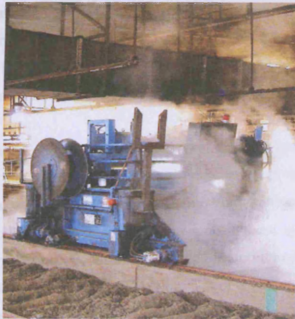
Figure 2.19. An example of an agitated bay composting system. The agitator moves along the top of the bay walls, lifting the organic waste and moving it a predetermined distance along the bay. (Composting Association, 2004).
