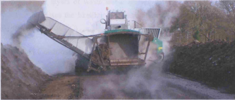
Figure 2.15. A self propelled windrow turner with a lateral turn device fitted. The lateral turn device uses conveyors to transfer the waste lifted by the turner further along the composting pad. This machine is capable of turning a windrow 5.7 meters wide and 2.8 meters high.
