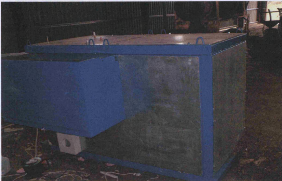
Figure 5.1 Highly insulated pilot scale in-vessel system.
