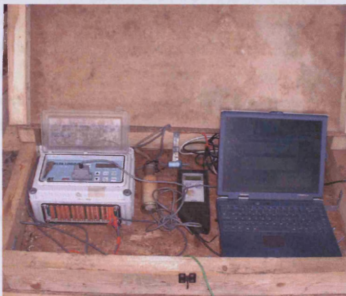
Figure 3.6. Data logger, moisture trap, moisture filter and gas analyser shown in secure box connected to the canopy, along with laptop computer used to download data.
