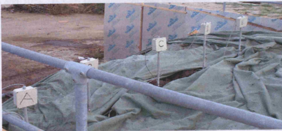
Figure 4.8 Thermocouple array inserted into compost at 0, 750, 1500, 2250 and 3000mm from the sidewall.
