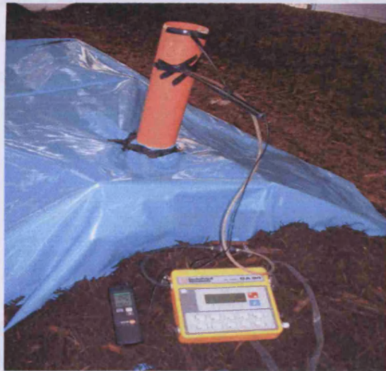
Figure 3.2. Temporary canopy channelling exhaust gases from a green waste windrow through a 110mm pipe. Hot wire anemometer used to measure velocity and infra red gas analyser to measure CO 2 concentration.
