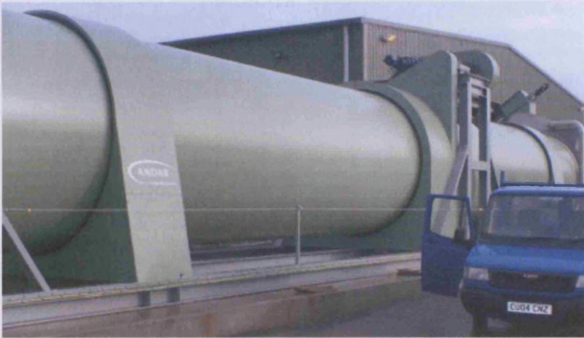
Figure 2.20. An example of a rotating drum composting system, it is approximately 30 meters long.
