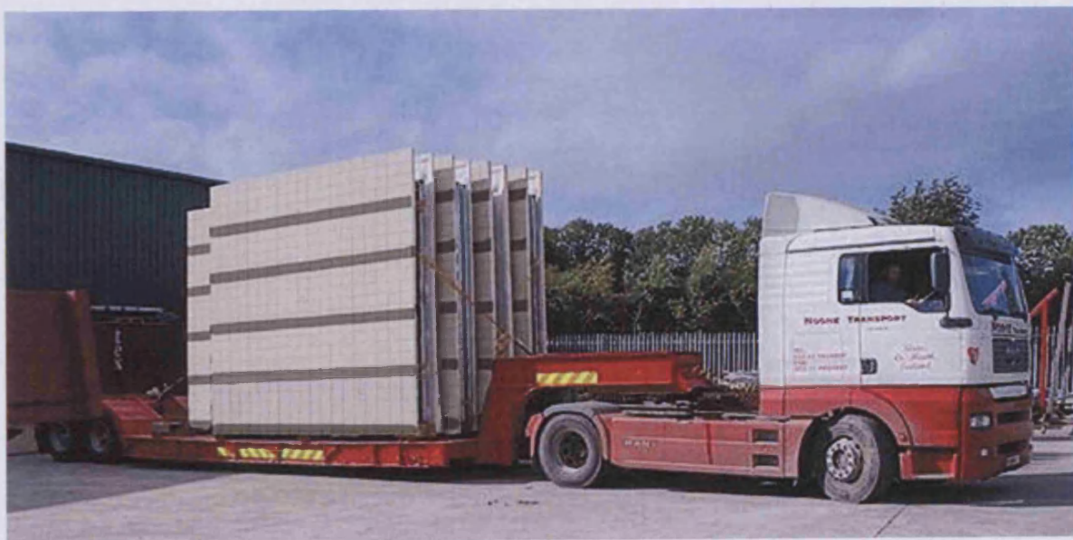
Figure 7-4: Closed panel system Source: (Kingspan Offsite, 2007)
