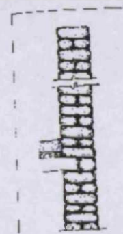
Figure (4-29) Section through the mud wall sun-dried mud brick ( labin ). Source: Mud Construction (4-21) .
