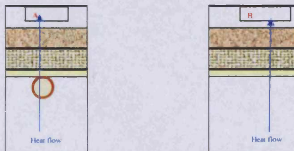
Figure (7-36) Heat flow ( U -value) for both sections in A and B.
