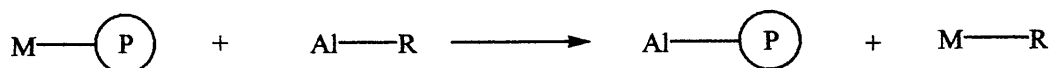
Scheme 5.1: Chain transfer to aluminium (M = Ti or Zr; R = alkyl ligand; P = polymer chain).
