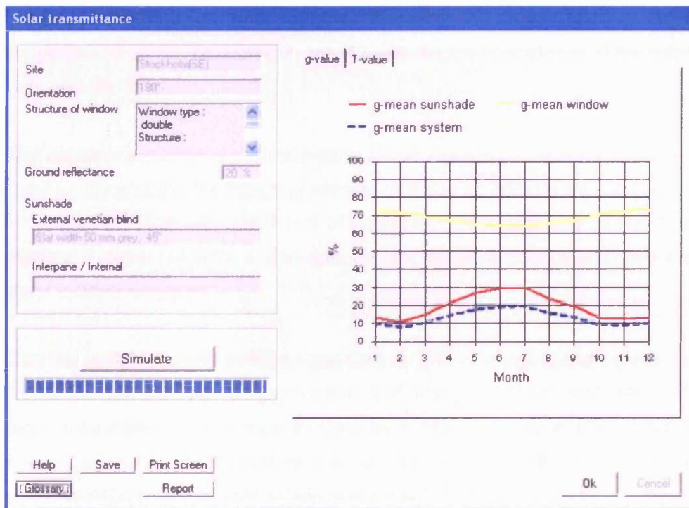
Figure 2.17: ParaSol, Solar Transmittance simulation output, © Division of Energy and Building Design, Department of Construction and Architecture, Lund Institute of Technology, Lund University
