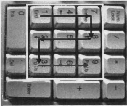
Figure 15. Numeric portion of keyboard (within white border) showing the first half of the key pressing sequence superimposed. The second part of the sequence was 9,8,7,4,5,6,3,2,1, after which the first part of the pattern repeated.
