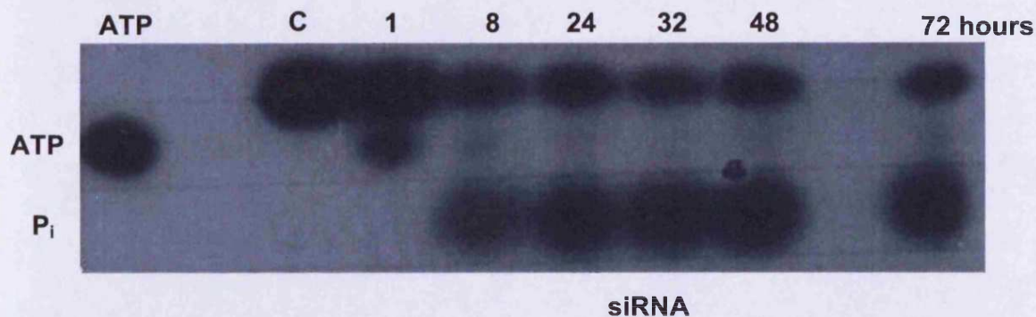
Figure 3.7: Stability assay in 10% FBS-containing media of radiolabelled siRNA. A 20% PAGE gel visualised by a phosphorimager shows a stability assay on siRNA in 10% FBS-containing D-MEM over 72 hours. ATP refers to free label gamma ^{32}\text{P} ATP run as a control. \text{P}_i is the suspected band for free phosphate. C= control siRNA, not exposed to degrading media that is equivalent in radioactivity to the other samples. The numbers on top refer to the time exposed to the media in hours.
