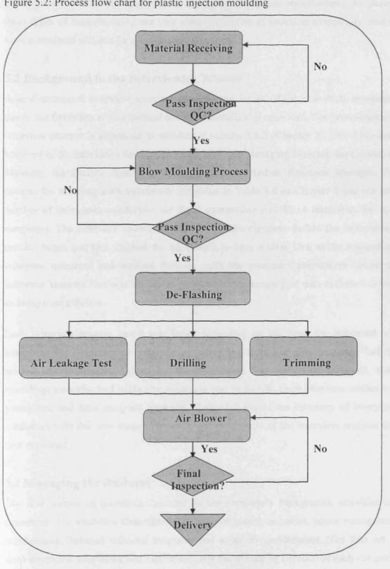
Figure 5.2: Process flow chart for plastic injection moulding
