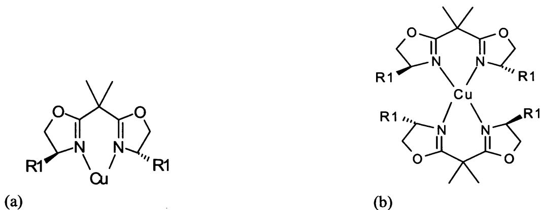
Figure 6: Sketch of Cu catalyst; (a) one bidentate bis(oxazoline) molecule is attached metal centre (Species B), (b) two bidentate ligands are attached (Species C)
