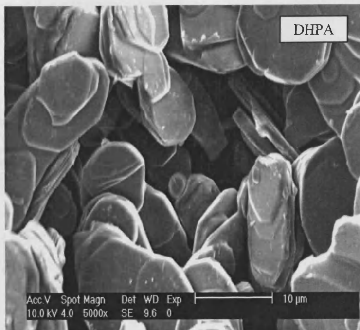
Fig. 4.6 The SEM of \text{VOPO}_4 \cdot 2\text{H}_2\text{O}
