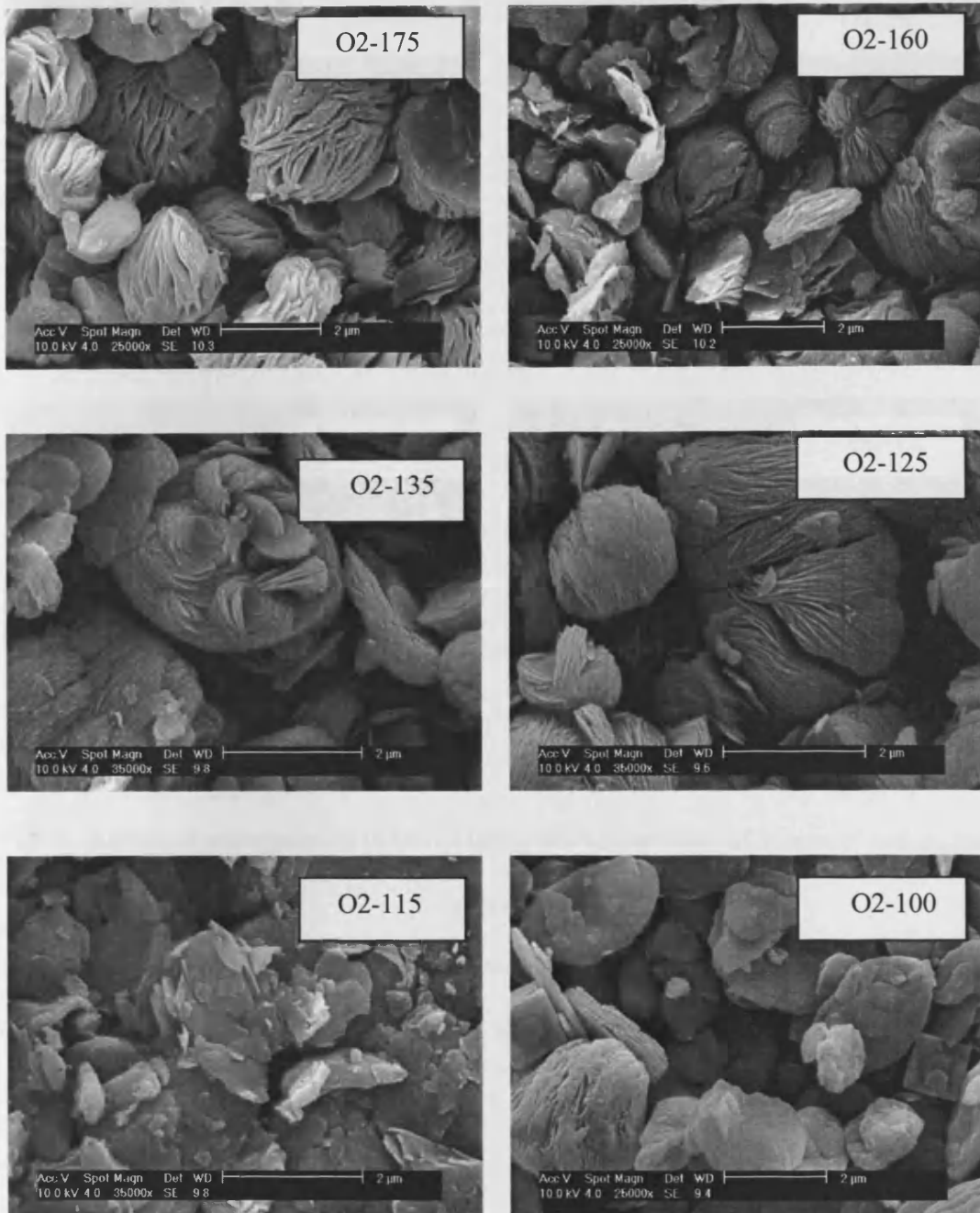
Fig. 3.12 SEM of new materials prepared using different amount of 1-octanol and octane solvent
