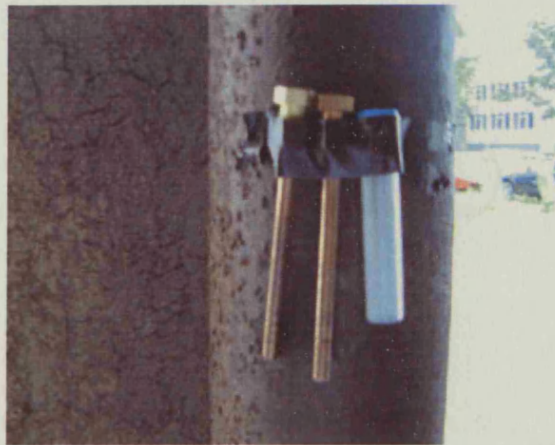
Figure 3.5 Passive Nitrogen dioxide, Nitrous oxide and BTEX tubes in place
