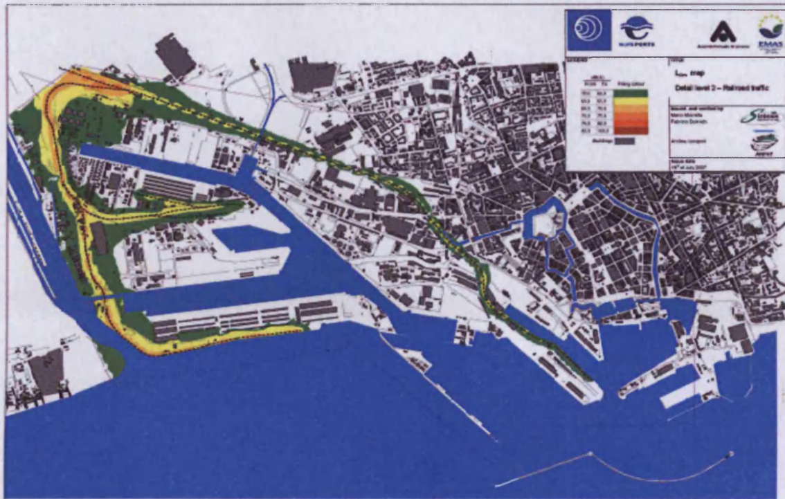
Figure 122: Port of Livorno – Railway traffic noise (Lden)
