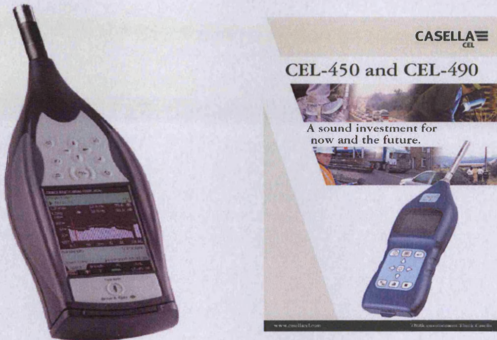
Figure 79: The Bruel & Kjaer 2250 (left) and the CASSELLA CEL-490 (right) Sound Level Meters
