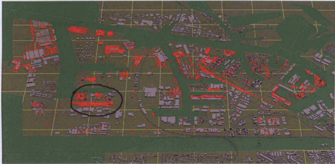
Figure 126: Initial noise model of the industrial area in the Port of Amsterdam
