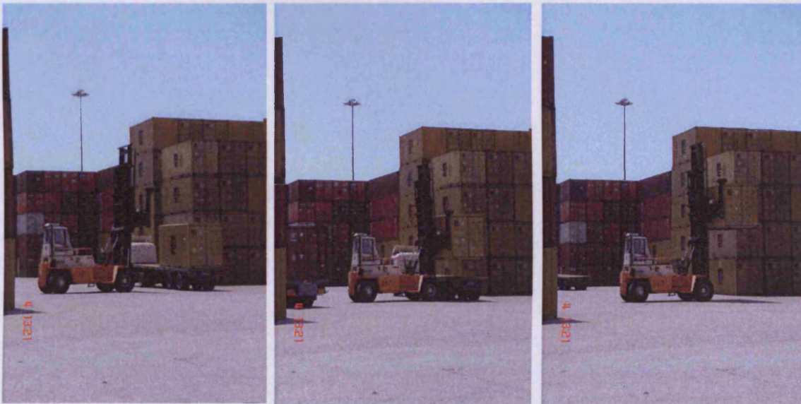
Figure 102: Empty containers handling with fork lifters
