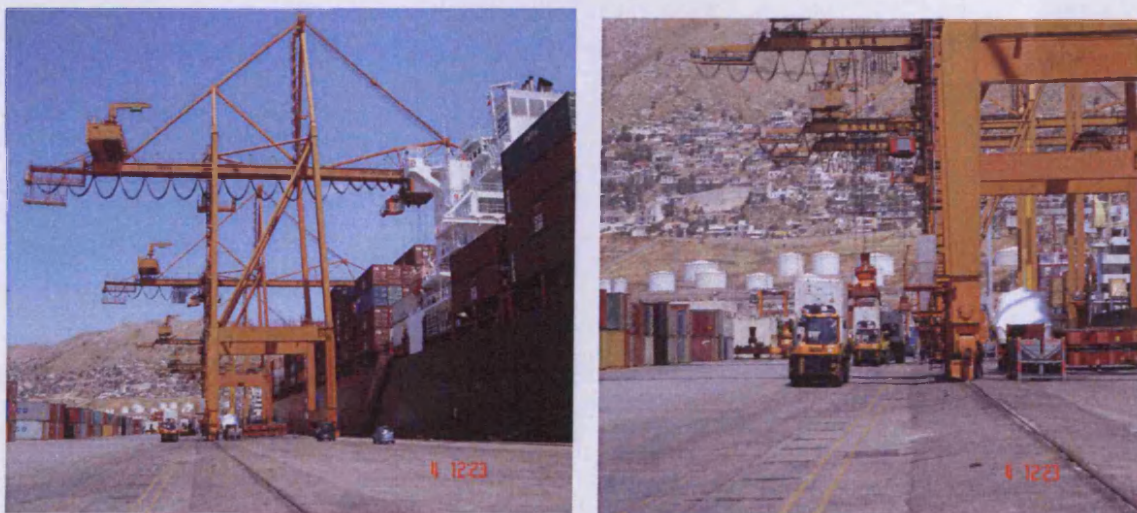
Figure 100: Loading – unloading container ships using container cranes
